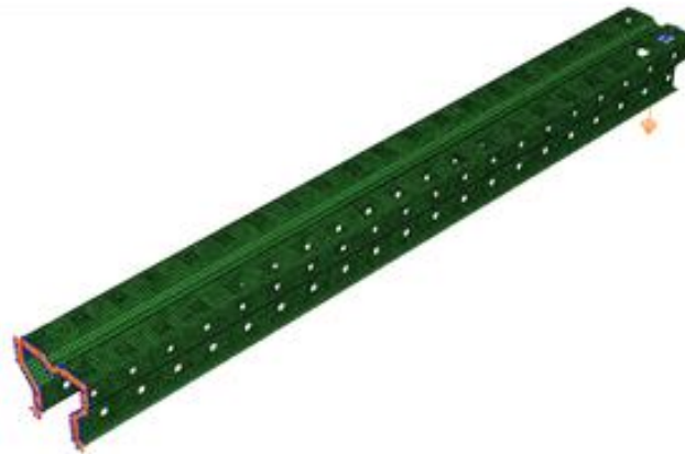
Fig. 10 Finite element model of upright section
