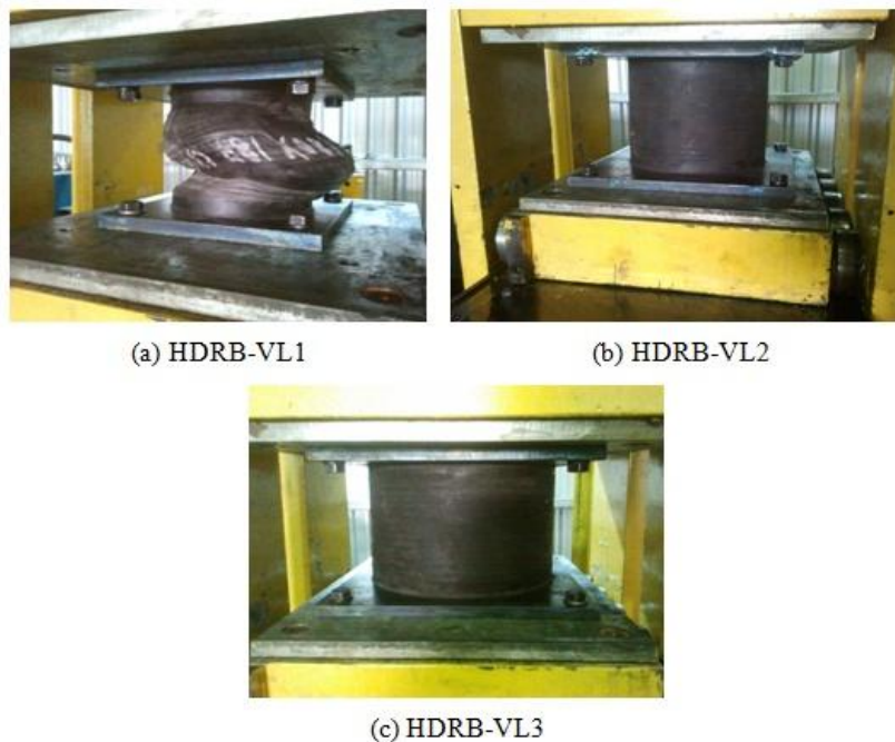
Fig. 6 Compression stiffness test of the three HDRB under designed loads
