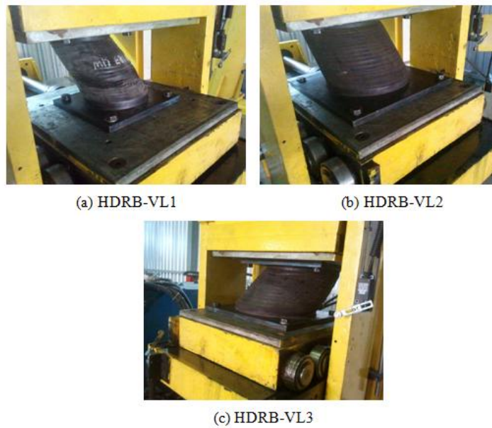
Fig. 9 Shear stiffness testing configuration of the three HDRB to \gamma = 150\%
