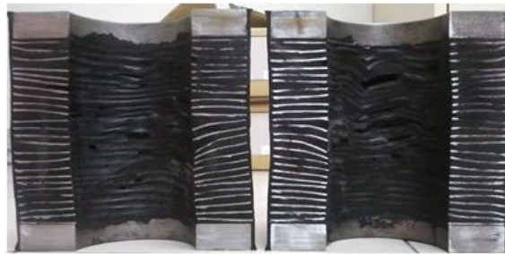
Fig. 8 Cross-sectional cut of HDRB-VL1 revealing bending of steel plates
