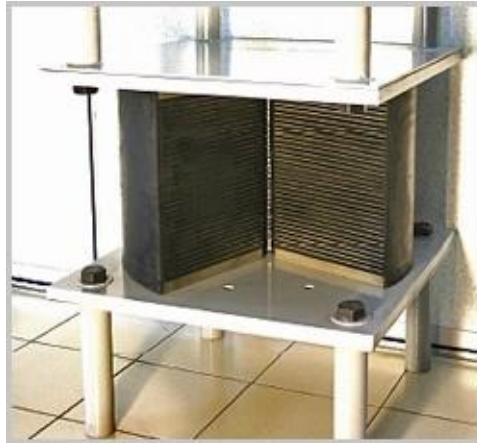
Fig. 1 High damping rubber bearing (HDRB) showing internal layers
