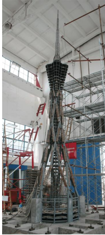
Fig. 2 Overview of the test model on shake table
