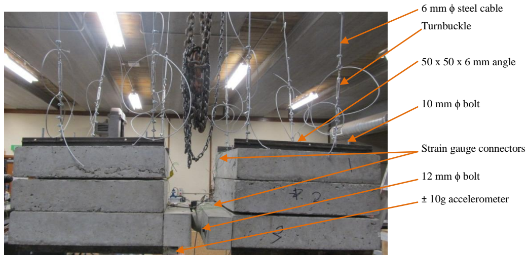
Fig. 3 Pounding with three concrete slabs on each pendulum (case s3-i3)
