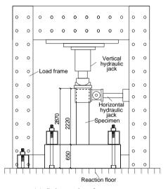
(a) Schematic of test setup
