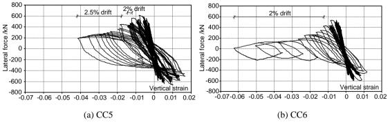
Fig. 13 Hysteresis loops of lateral force versus vertical strain for plastic hinge of specimens
