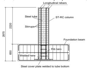
(d) Elevation view of steel tube and reinforcement Fig. 2 ST-RC column specimens (unit: mm)
