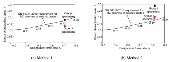
Fig. 4 Design axial force ratio versus stirrup characteristic value of specimens
