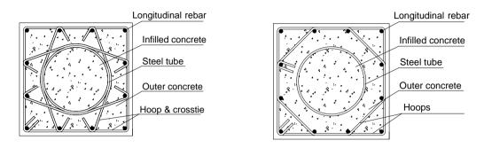
Fig. 1. Steel tube-reinforced concrete (ST-RC) composite column
