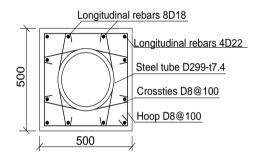
(b) Section dimensions and reinforcement details for Group I specimens: CC1, CC3, CC5
