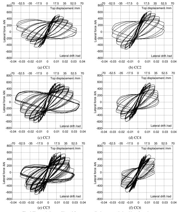
Fig. 9 Hysteretic loops of lateral force versus displacement relationships of specimens
