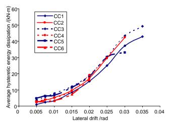
Fig. 14 Curves of average hysteretic energy dissipation versus drift ratio
