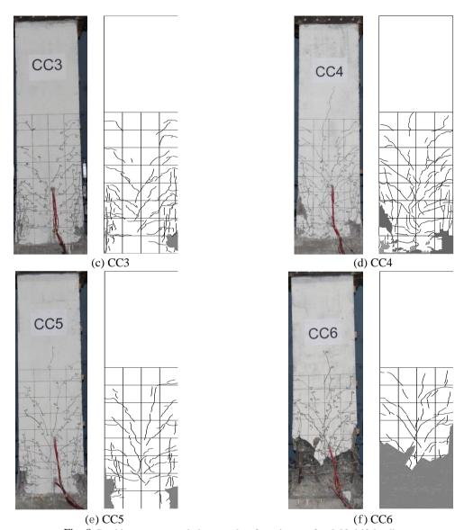
Fig. 8 Cracking patterns and photographs of specimens after 0.02 drift loading
