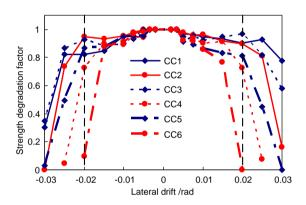
Fig. 16 Degradation of flexural strength of specimens
