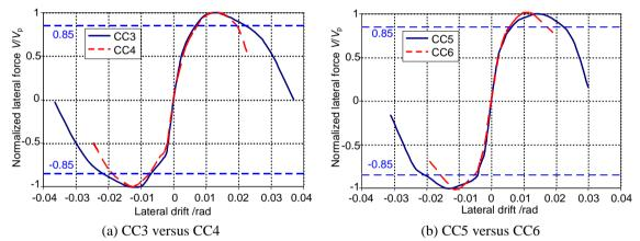
Fig.12 Envelope curves of normalized lateral force versus drift ratio: Effect of amount of transverse reinforcement
