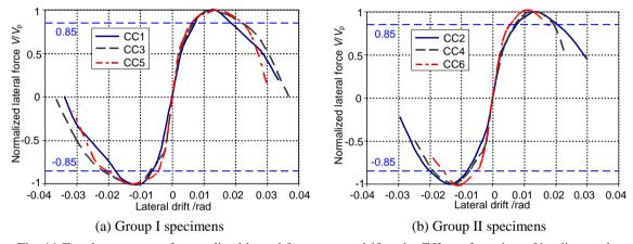
Fig. 11 Envelope curves of normalized lateral force versus drift ratio: Effect of number of loading cycles
