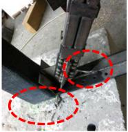
(c) Uplift of column and buckling of T angle
