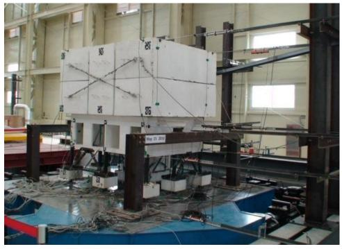
Fig. 11 Overview of earthquake simulation test set up of the model strengthened with BRB's and FRP
