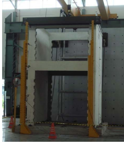
Fig. 3 Full scale HCPS model for lateral cyclic loading test
