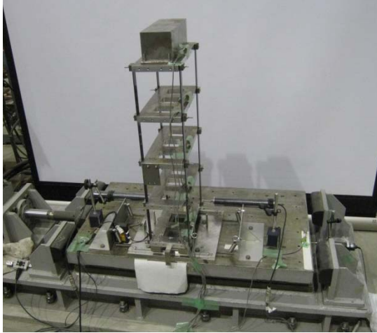
Photo 1 Four-story base-isolated test structure
