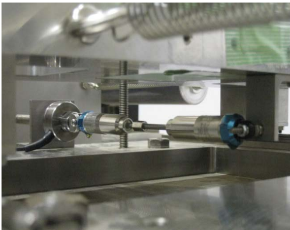
Photo 2 Mini piston as viscous damper
