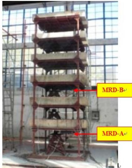
Fig. 2 Photograph of the tested structure with MR dampers
