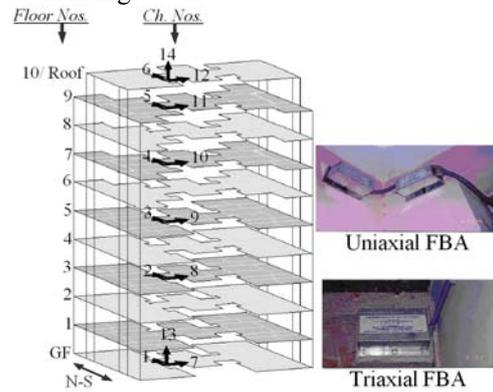
Fig. 2(b) locations of sensors at various floors and channel numbers
