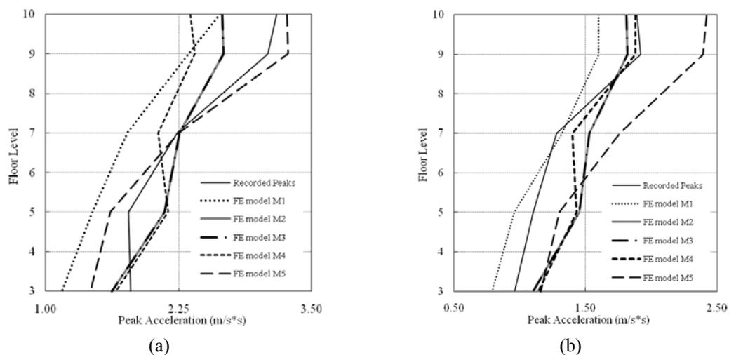
Fig. 10 Peak absolute accelerations, recorded and from FE models in (a) N-S direction and (b) E-W direction
