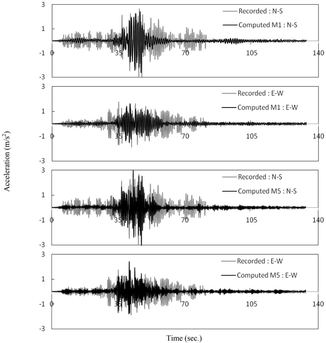
Fig. 9 Recorded and computed time history at 10<sup>th</sup> floor of FE model M1 and M5
