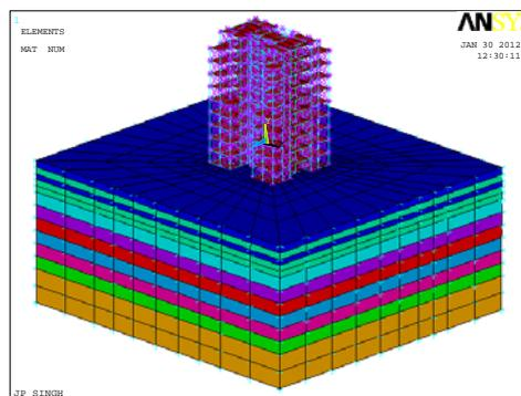
Fig. 8 FE model of Building-Raft-Soil System (M6)
