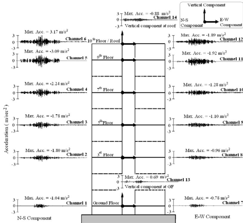
Fig. 4 Corrected acceleration time histories and the peak value of accelerations at various floors of RPOSQ building
