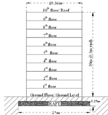
Fig. 1(b) Elevation in N-S direction of RPOSQ building
