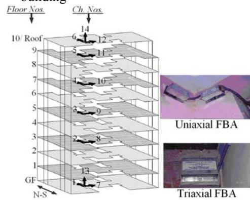
Fig. 2(b) locations of sensors at various floors and channel numbers
