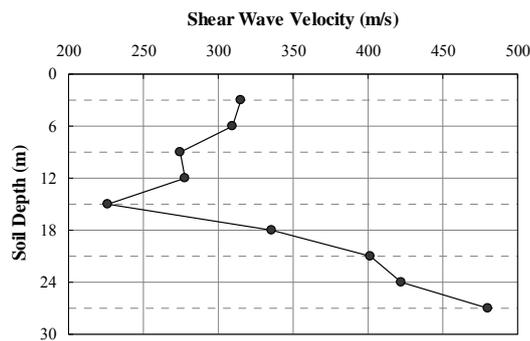
Fig. 3 Shear wave velocity at vertical points from cross borehole tests
