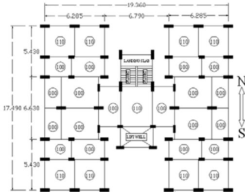
Fig. 2(a) Typical plan of upto 5<sup>th</sup> floor level, orientation of columns and thickness of floor slabs
