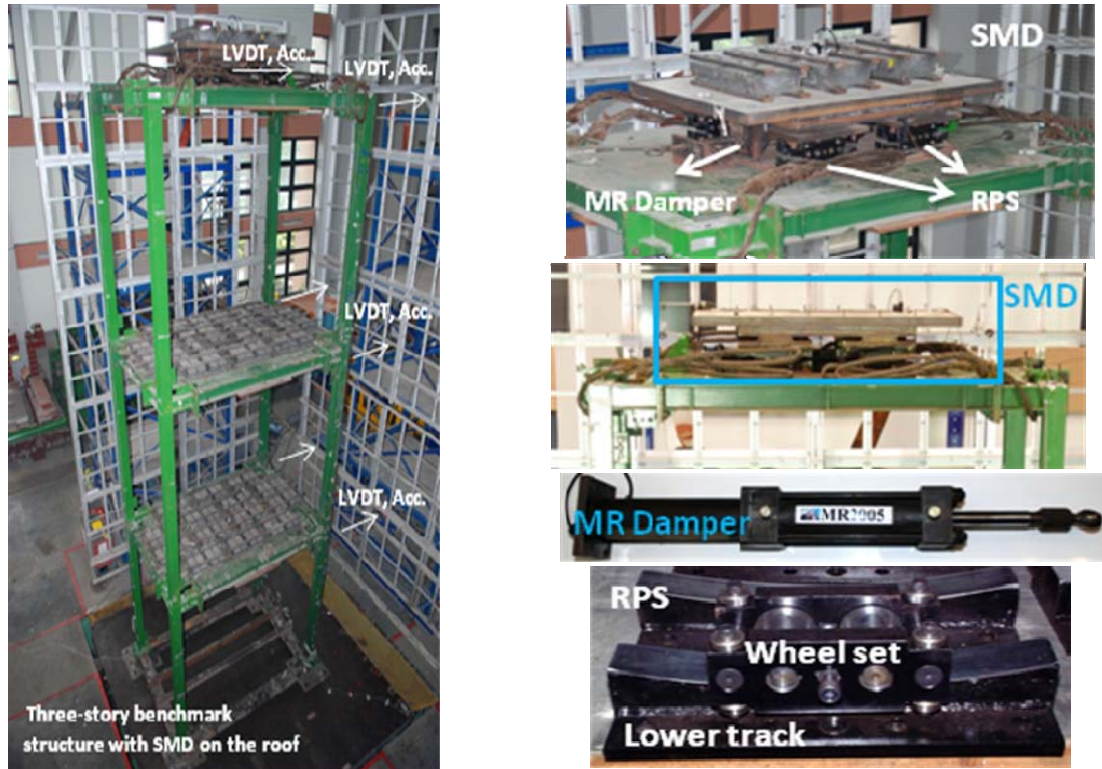
Fig. 9 Set-up of the three-story benchmark structure
