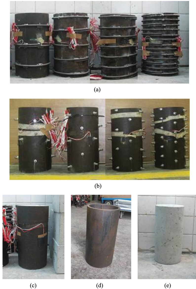
Fig. 1 Photos of the test specimens: (a) CFST columns with steel rings ( s = 20t , 15t , 10t and 5t ), (b) CFST columns with steel ties ( s = 20t , 15t , 10t and 5t ), (c) CFST column without external confinement, (d) hollow steel tube and (e) plain concrete cylinder
