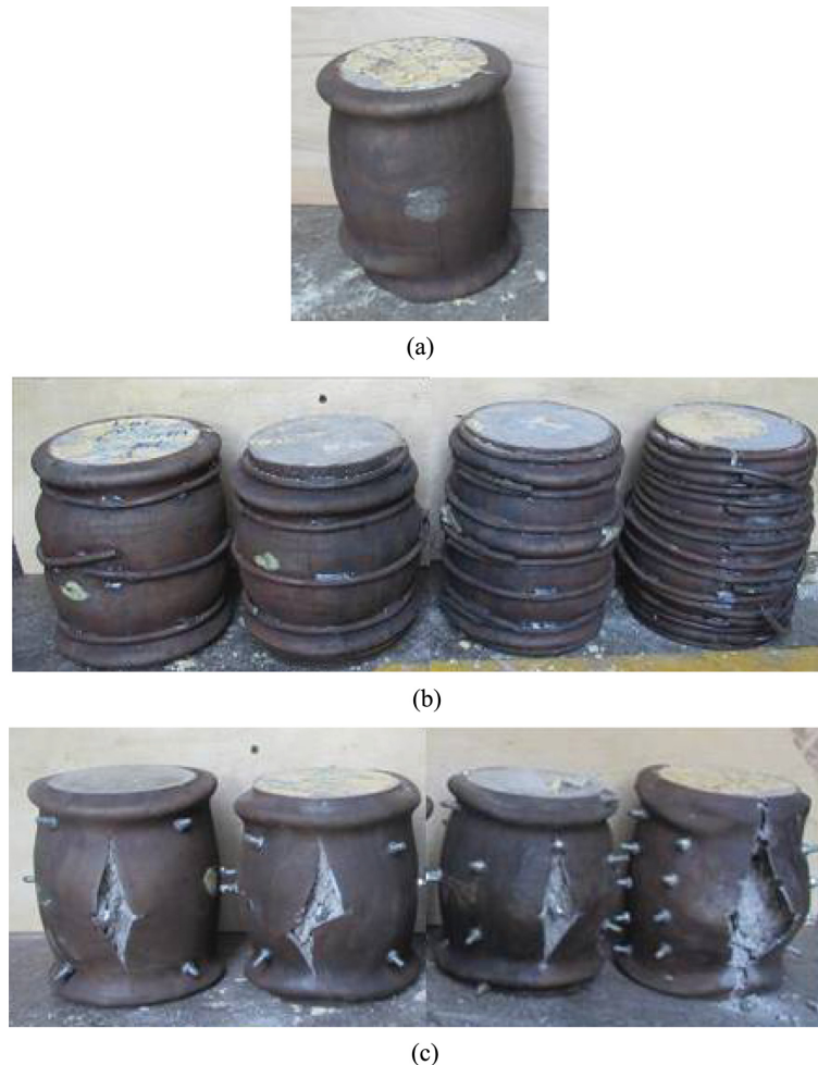
Fig. 9 Photos of CFST columns: (a) CFST column without external confinement (30-5-00X), (b) ring-confined CFST columns ( s = 20t, 15t, 10t and 5t ) and (c) tie-confined CFST columns at failure ( s = 20t, 15t, 10t and 5t )
