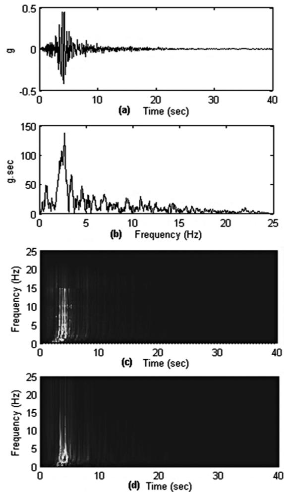
Fig. 10 Loma Prieta earthquake: (a) acceleration, (b) Fourier transform, (c) CWT by proposed method and (d) CWT by *db2*
