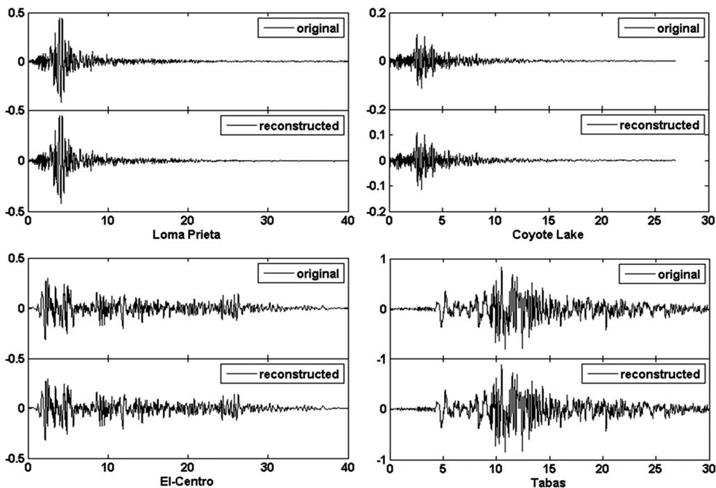
Fig. 6 Original and reconstructed earthquakes using proposed method
