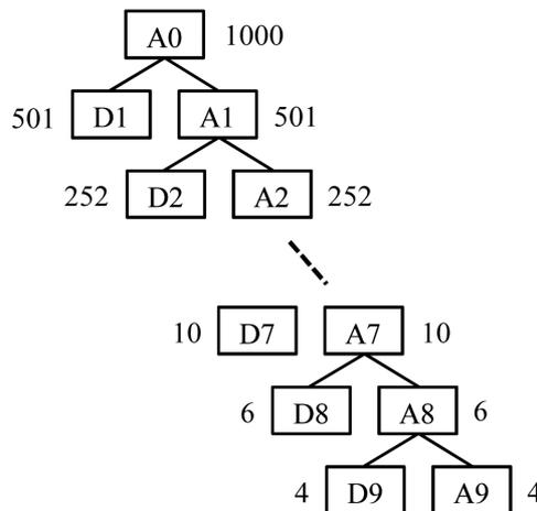
Fig. 1 Wavelet decomposition tree for a 1000 sample point signal
