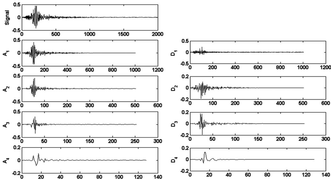
Fig. 7 Decomposition tree for Loma Prieta earthquake using the proposed method
