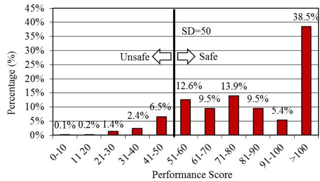
Fig. 13 The distribution of the inspected buildings according to earthquake performance score for SD=50
