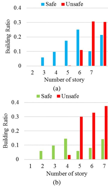
Fig. 22 Safe and unsafe building ratio according to the heavy overhangs: (a) SD=50 (b) SD=60
