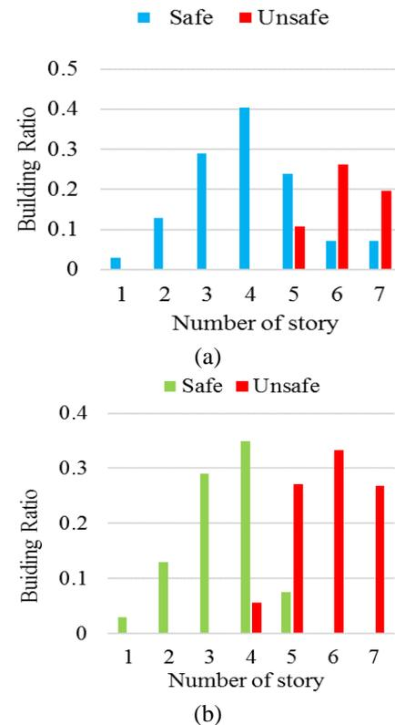
Fig. 23 Safe and unsafe building ratio according to the soft-story: (a) SD=50 (b) SD=60
