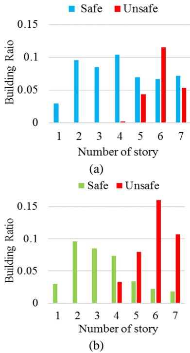
Fig. 24 Safe and unsafe building ratio according to the short-column: (a) SD=50 (b) SD=60
