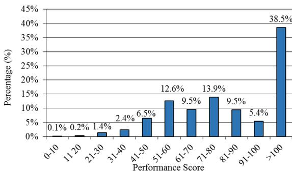
Fig. 11 The distribution of the inspected buildings according to the earthquake performance score
