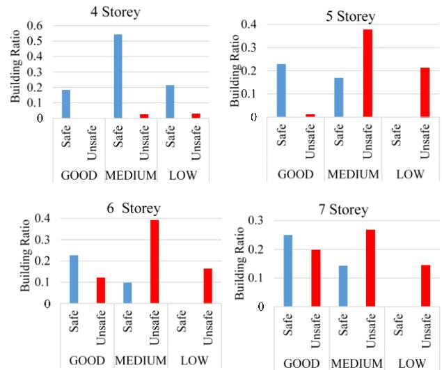
Fig. 26 Safe and unsafe building ratio according to the visual quality for SD=60
