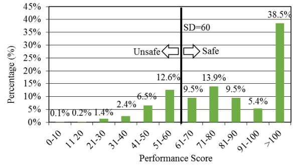
Fig. 17 The distribution of the inspected buildings according to earthquake performance score for SD=60
