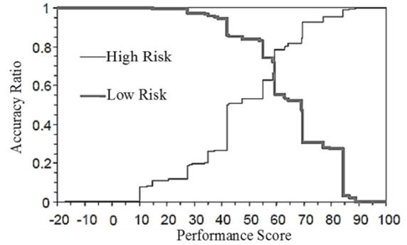
Fig. 12 The relationship between the accuracy ratio and the calculated earthquake performance score based on the Duzce earthquake database (Sucuoglu 2007)
