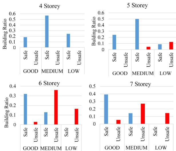
Fig. 25 Safe and unsafe building ratio according to the visual quality for SD=50
