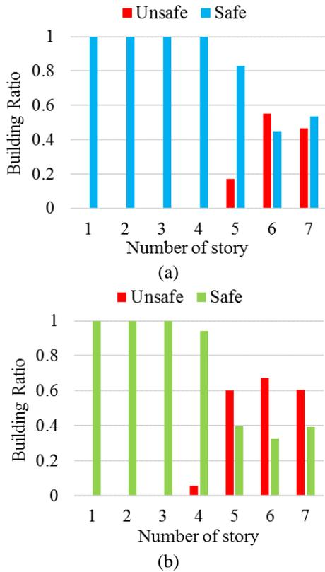
Fig. 21 Safe and unsafe building ratio according to the number of story: (a) SD=50 (b) SD=60
