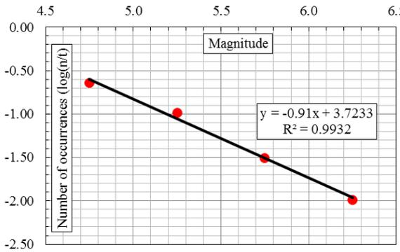
Fig. 4 Relation between the magnitude and the frequency of the earthquake
