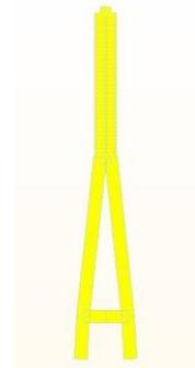
Fig. 5 The lateral configuration of inverse Y-shaped tower
