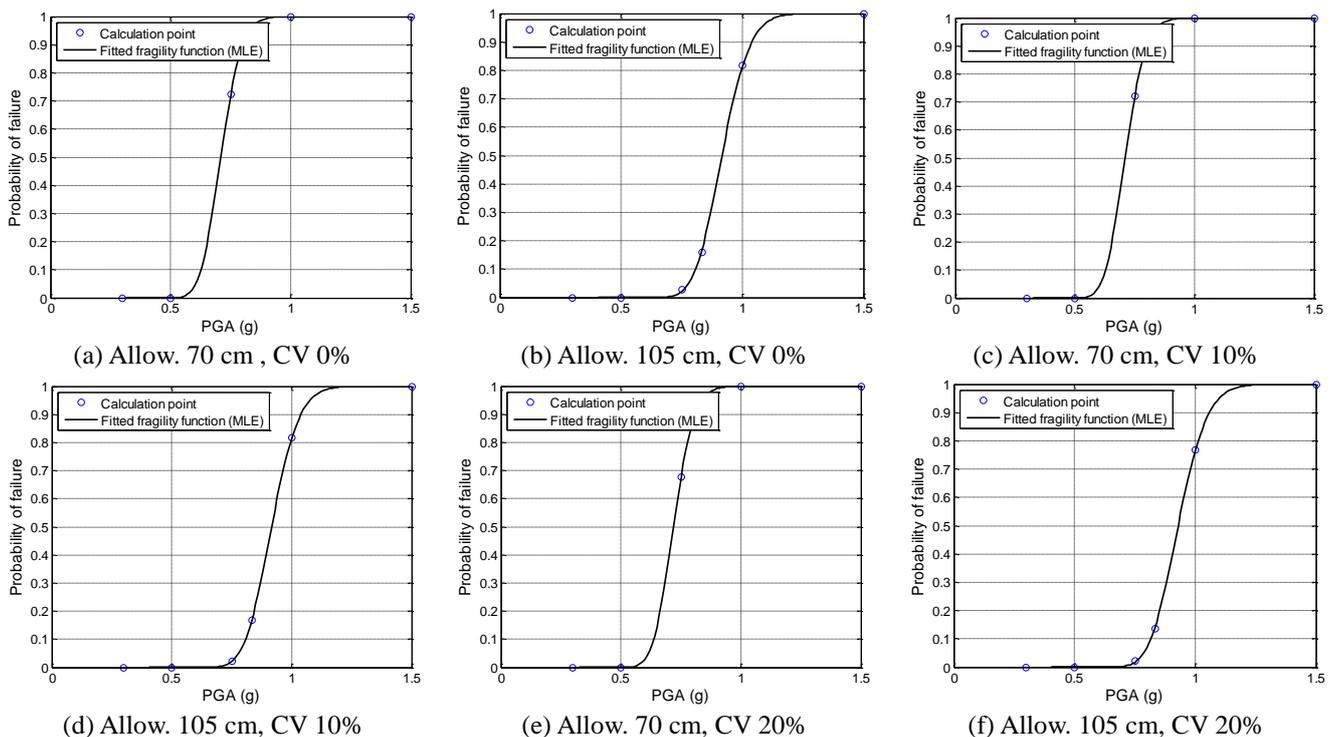
Fig. 10 The fragility curve of isolated nuclear power plant
