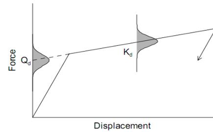
(a) Mechanical properties of the isolation system (Huang *et al.* 2009)
