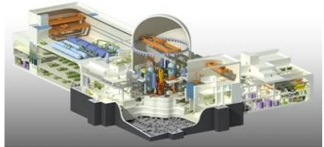
Fig. 8 Concept of base-isolated Advanced Power Reactor 1400 (KEPCO E&C 2012)
