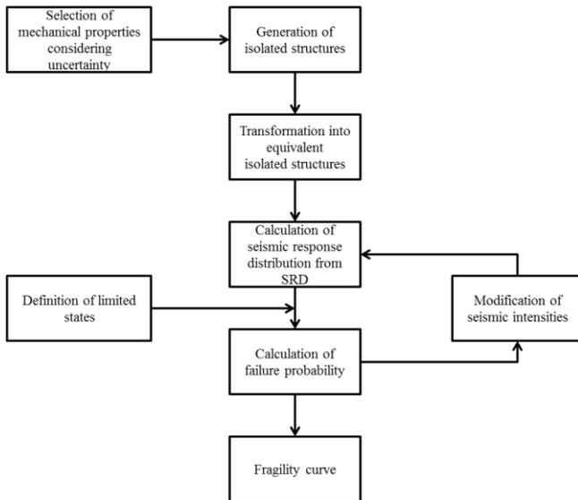
Fig. 6 Flowchart of fragility assessment for isolated structures using the SRD
