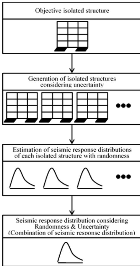
Fig. 2 Flowchart of calculating the seismic response distribution
