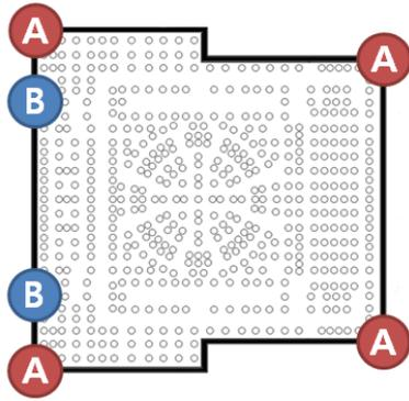
Fig. 9 Location of the edge of the isolated structure (A) and main pipelines (B) and dispositions of isolators
