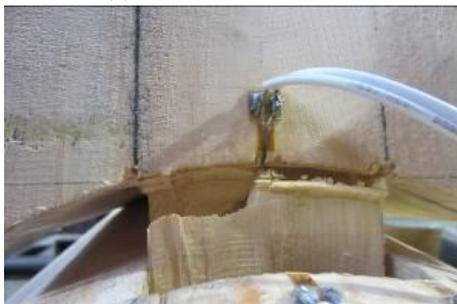
(b) Tensile failure of the tenon-neck
