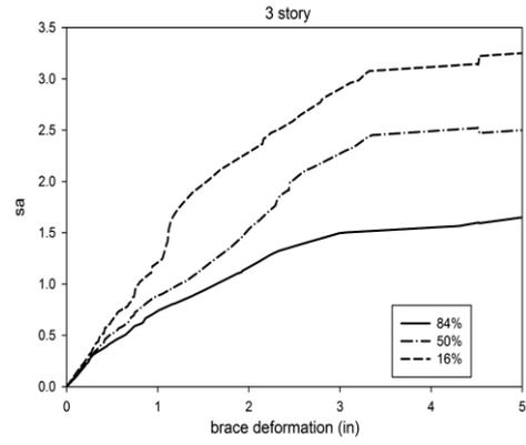
Fig. 9 Compact IDA curves for BRBF-3 story structure
