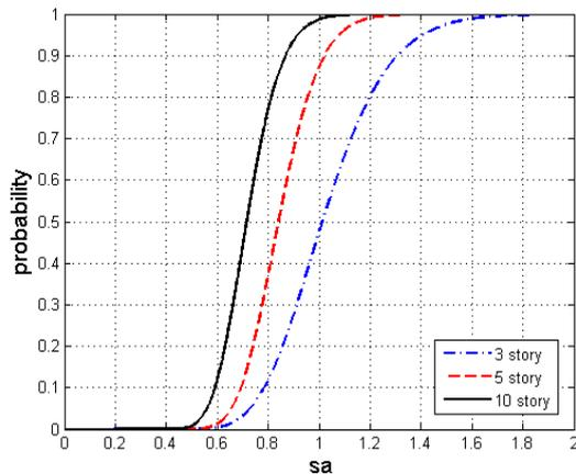
Fig. 16 Fragility curves at CP level for SCBF system
