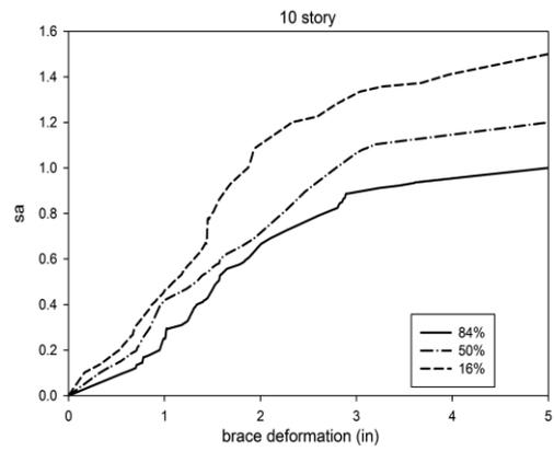
Fig. 11 Compact IDA curves for BRBF-10 story structure
