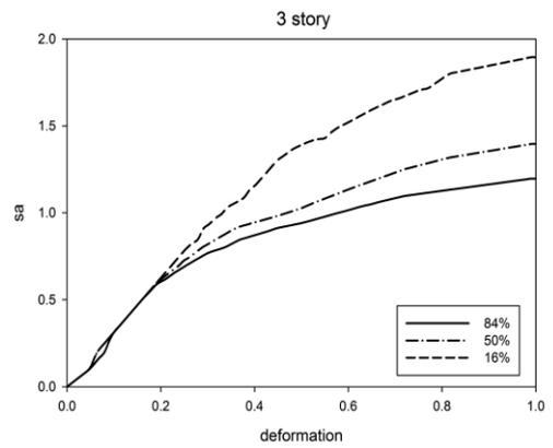
Fig. 12 Compact IDA curves for SCBF-3 story structure
