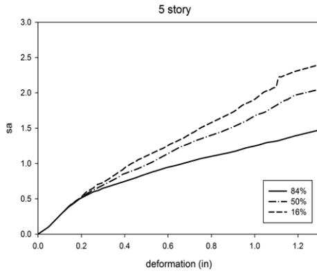
Fig. 13 Compact IDA curves for SCBF-5 story structure
