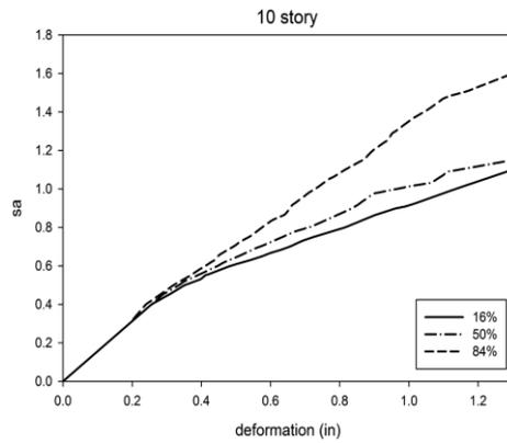
Fig. 14 Compact IDA curves for SCBF-10 story structure
