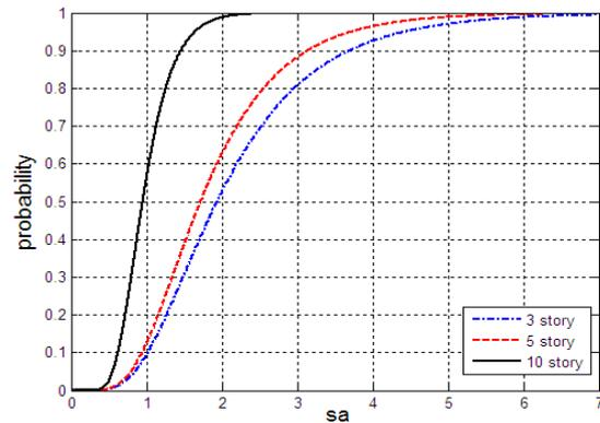
Fig. 15 Fragility curves at CP level for BRBF system
