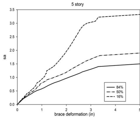
Fig. 10 Compact IDA curves for BRBF-5 story structure
