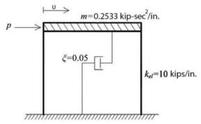
Fig. 7 A SDOF system with nonlinear behavior
