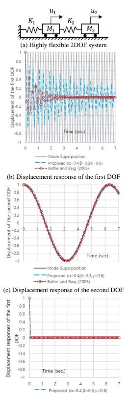
(d) Displacement response of the first  $DOF(K_1=10^7)$ Fig. 2 Weak instability assessment of the proposed method through solving a highly flexible system
