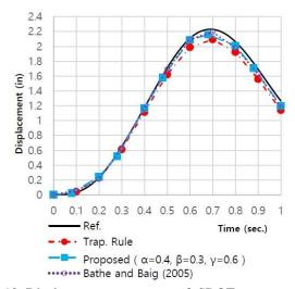
Fig. 10 Displacement responses of SDOF system under dynamic loading
