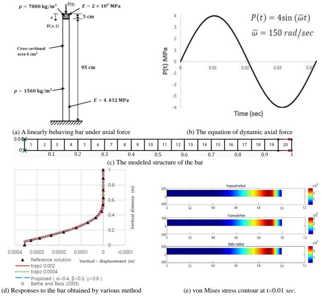
Fig. 6 First Example: the bar under dynamic axial load
