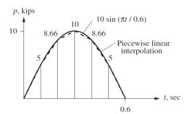
Fig. 9 The harmonic load acting on the system (Chopra 2007)
