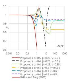
Fig. 1 Spectral Radius as a function of  $\Delta t/T$
