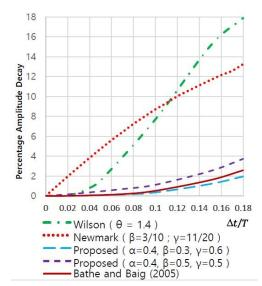
Fig. 3 Percentage numerical damping versus  $\Delta t/T$
