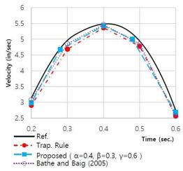
Fig. 11 Velocity responses of SDOF system under dynamic loading
