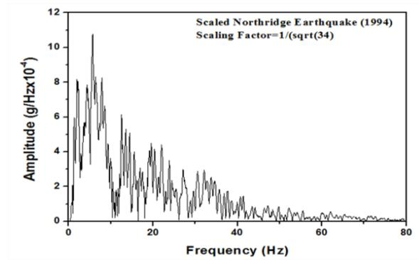
(b) Fourier transform for Northridge Earthquake
