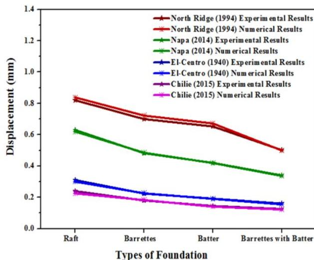
Fig. 7 Comparison of maximum displacement values of numerical and experimental work for different earthquakes
