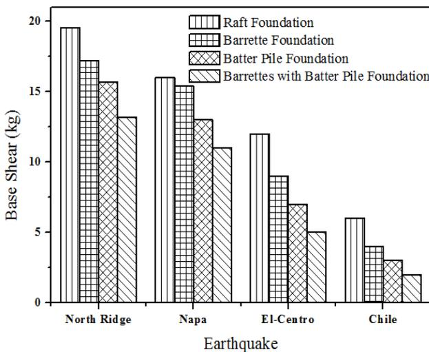
Fig. 13 Base shear for turbo generator foundation with raft, with barrette, with batter Pile and barrettes with batter pile obtained from computational analysis in SAP 2000
