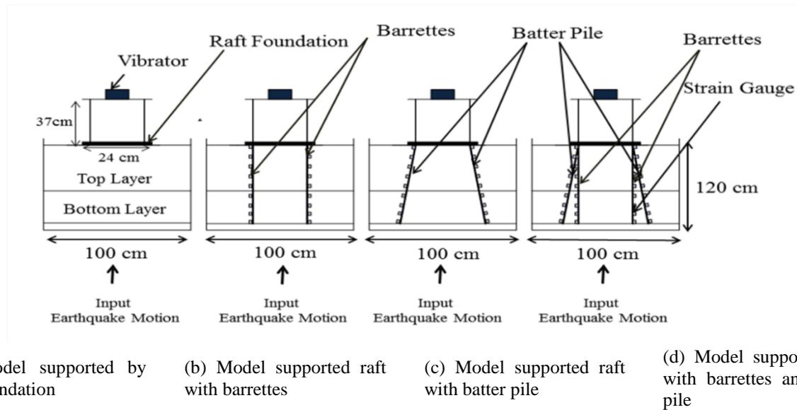
Fig. 3 Line diagram of the experimental model
