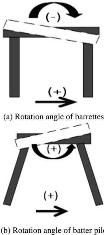
Fig. 12 comparison of rotation angle of barrettes and batter piles
