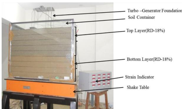
Fig. 2 Turbo generator foundation model with shaking table experiment
