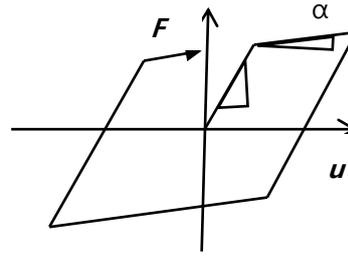
Fig. 1 (b) The force deformation behaviour of the nonlinear spring
