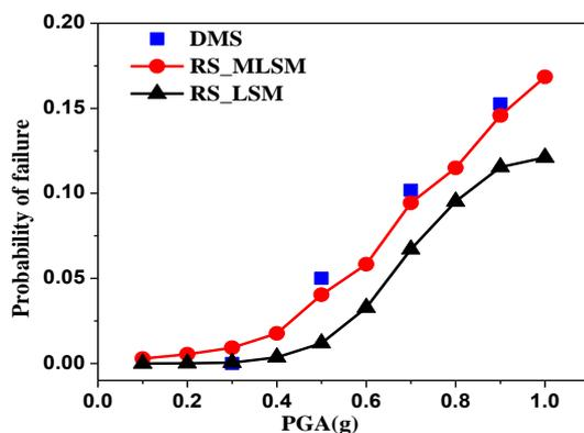
Fig. 10 The Comparison of fragility curves of the considered building frame at LS level
