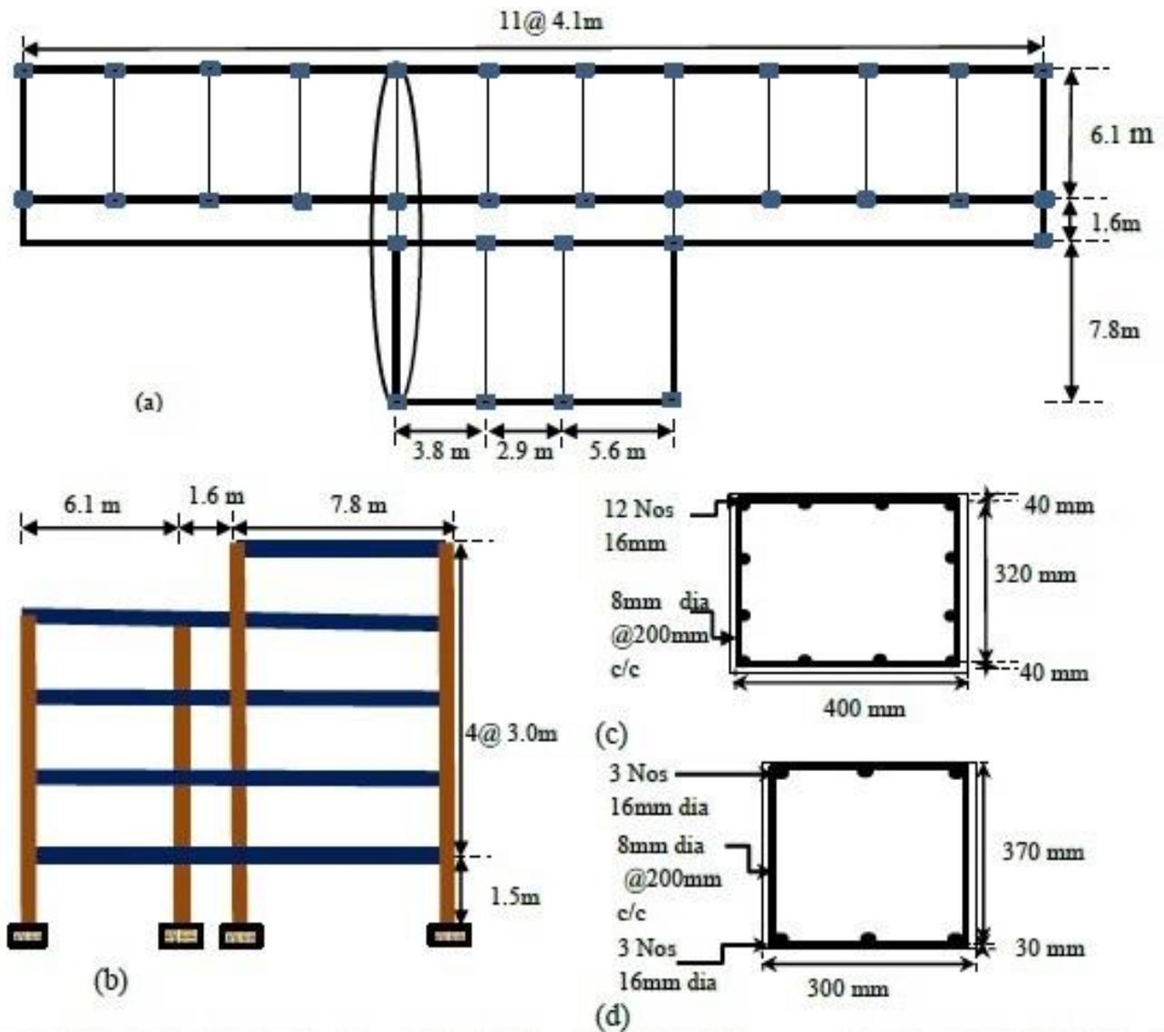
Fig. 7 The details of the building frame (a) the building plan, (b) the 2D frame, (c) the details of the column sections and (d) the details of the beam sections considered for SFA
