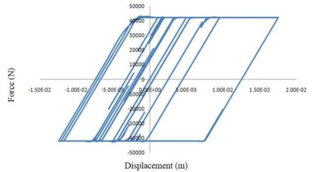
Fig. 3 The hysteretic behavior of CFDs in the first floor of 4-story frame
