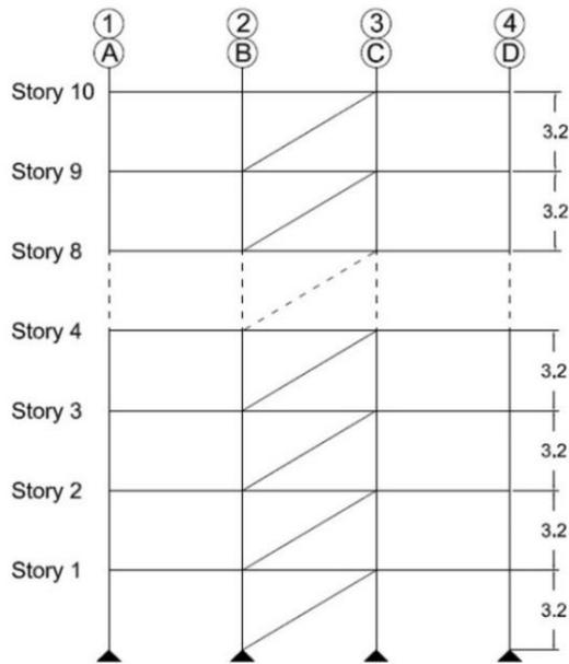
Fig. 2 The elevation of 2D frames modeled in OpenSees (dimensions in meter)
