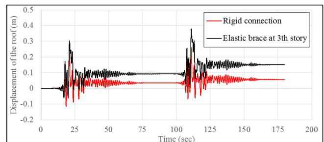
Fig. 6 Displacement time-history response of the roof for 6-story frame under San Simeon CA equipped with CFD (slip load of 20% of the story weight)
