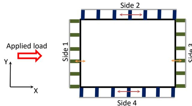
Fig. 7 Plan view of Configuration of shear and axial behaviour of façade brackets in building structure during earthquake
