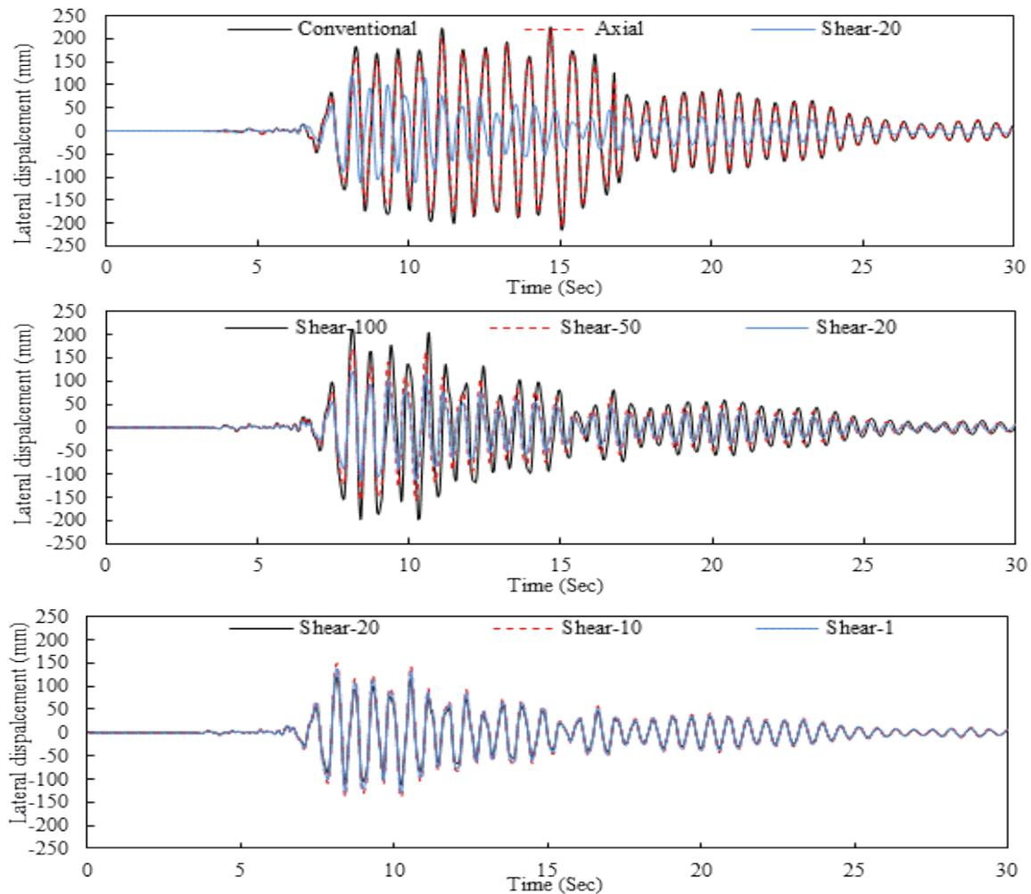
Fig. 9 Top displacements of primary structure coupled with DSFs with different bracket connector stiffness during 1995 Kobe Earthquake
