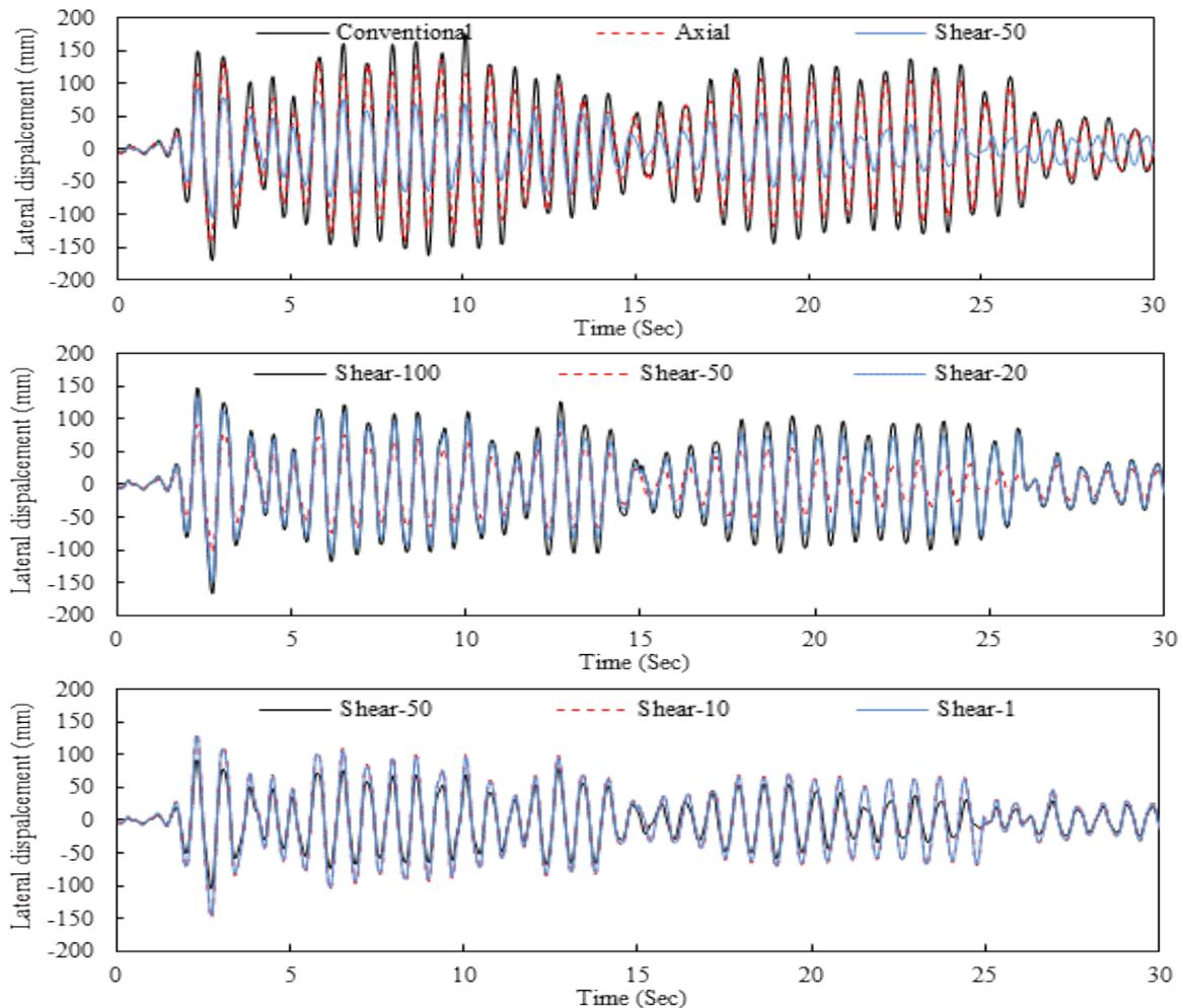
Fig. 8 Top displacements of primary structure coupled with DSFs with different bracket connector stiffness during 1940 El-Centro Earthquake
