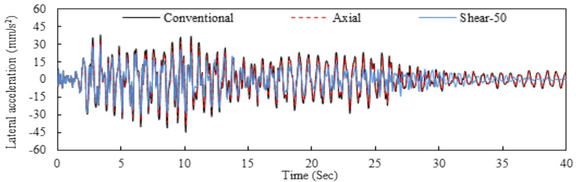
Fig. 12 Time-history top floor accelerations (mm/sec<sup>2</sup>) of primary structure coupled with DSFs with optimal bracket connector stiffness during 1940 El-Centro Earthquake
