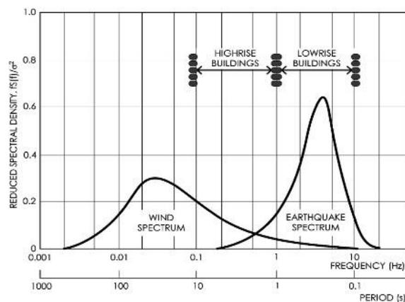
Fig. 1 Seismic and wind hazard versus excitation frequency (or period)
