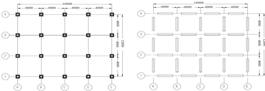
Fig. 5 Plan view of the 3-D frame model (dimensions are in mm)
