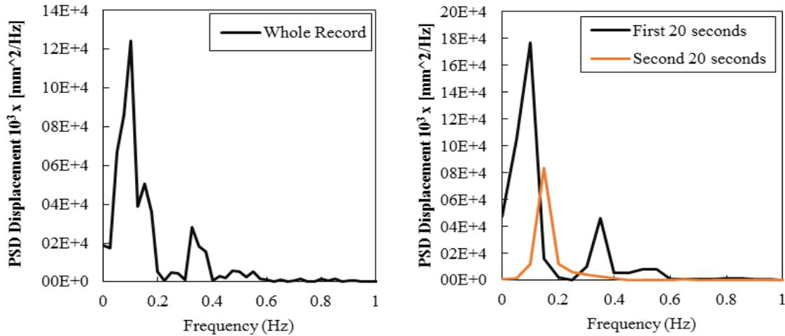
Fig. 2 Displacement Power Spectral Density for 1940 El-Centro earthquake
