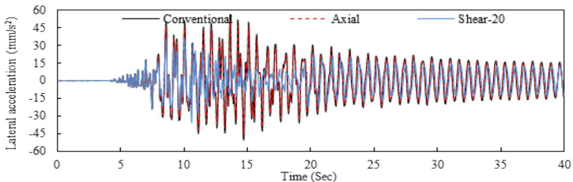
Fig. 13 Time-history top floor accelerations (mm/sec<sup>2</sup>) of primary structure coupled with DSFs with optimal bracket connector stiffness during 1995 Kobe Earthquake
