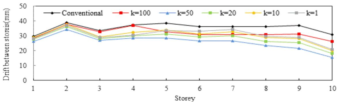
Fig. 10 Drift for primary structure with different stiffness for shear bracket façade elements during 1940 El-Centro earthquake
