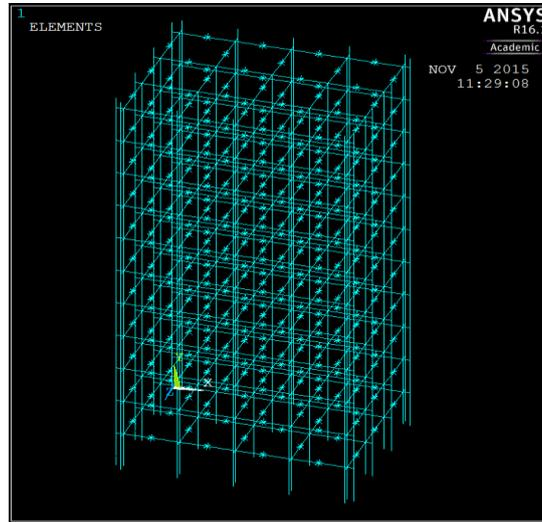
Fig. 4 Front view of exterior elevation of the 3-D frame model
