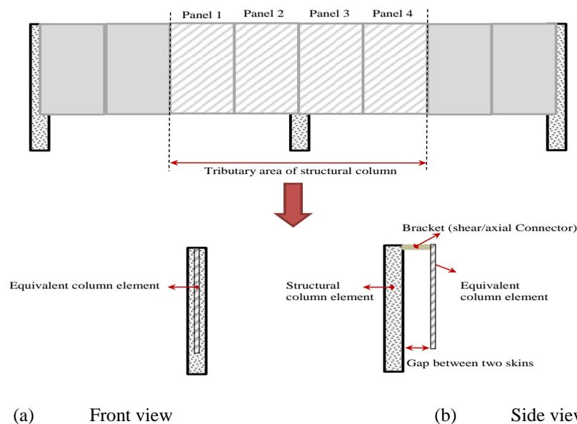
Fig. 6 Schematic view of facade column element and its configuration in each floor
