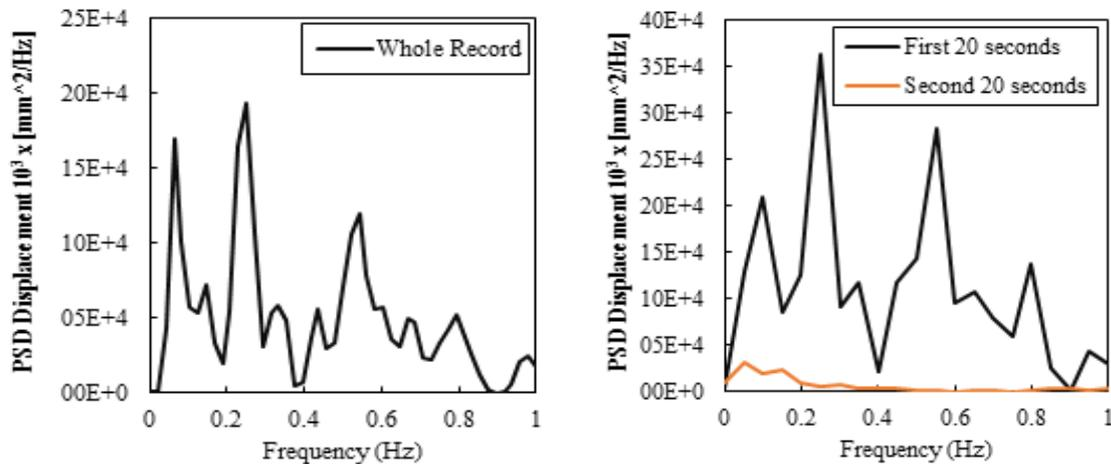
Fig. 3 Displacement Power Spectral Density for 1995 Kobe earthquake
