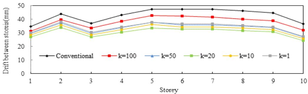
Fig. 11 Drift for primary structure with different stiffness for shear bracket façade elements during 1995 Kobe earthquake
