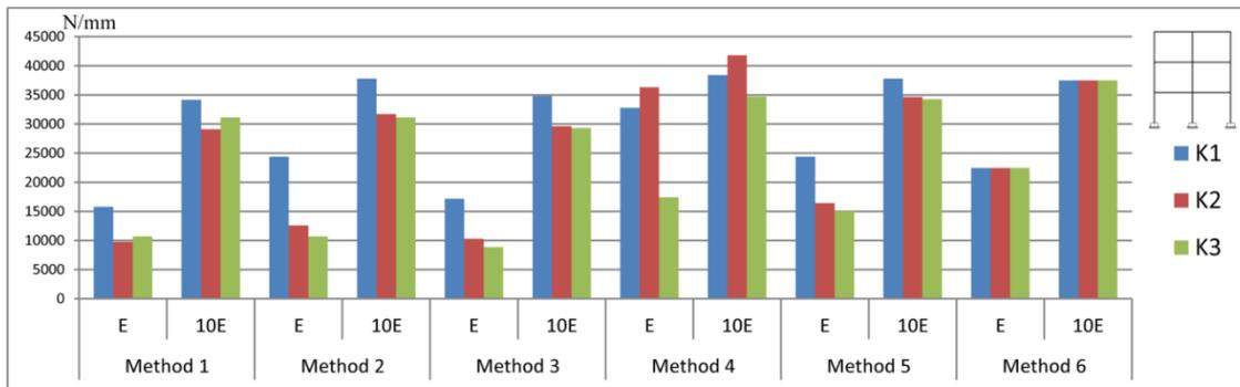
Fig. 12 Stiffness of three-storey frames with width of beams equal to columns and rigid supports in two types of Young's modulus of beams equal to columns and ten times the columns
