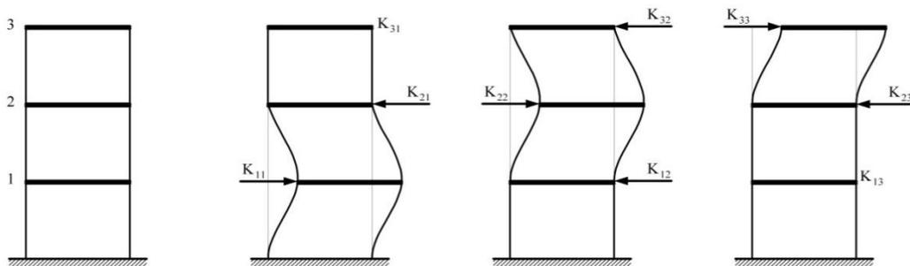
Fig. 17 Finite element model for calculating the storey stiffness
