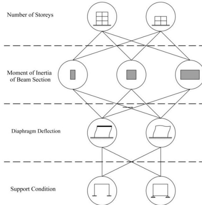
Fig. 8 Four variables and 24 types of frame to study calculation methods of Storey Stiffness
