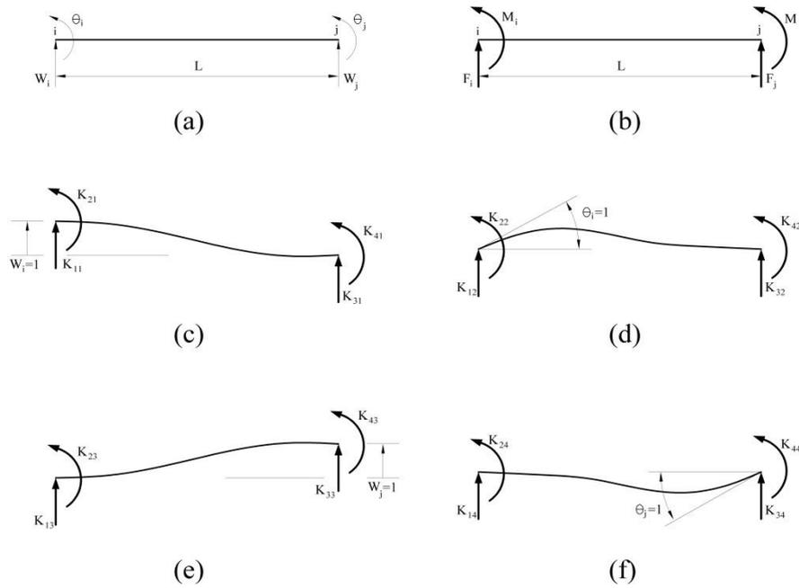
Fig. 16 (a) Four nodal degrees of freedom of a uniform beam, (b) Nodal force and moment, (c-f) Translational and rotational stiffness of each nodal degrees of freedom of a uniform beam
