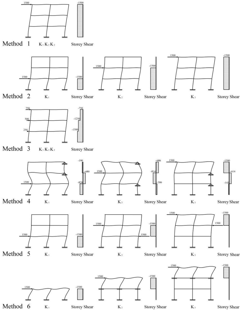
Fig. 7 Six accurate calculation methods of Storey Stiffness
