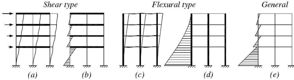
Fig. 4 Lateral displacement shape and moment distribution in shear and flexural models; (a) Lateral displacement of shear model, (b) Moment distribution of shear model, (c) Lateral displacement of flexural model, (d) Moment distribution of flexural model, (e) Moment distribution of flexural-shear model (Caterino *et al.* 2013)
