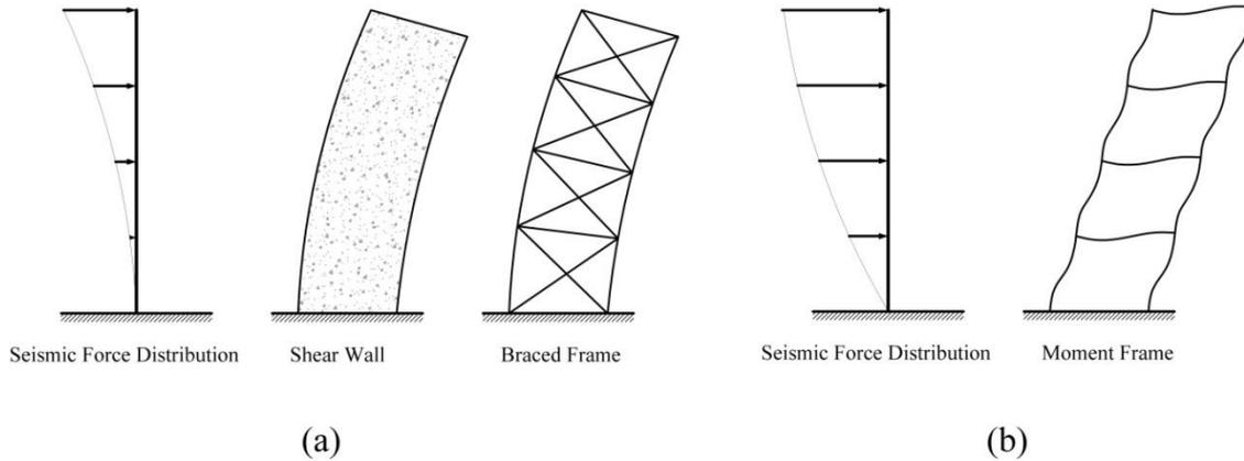
Fig. 3 Seismic force distribution and lateral displacement of structures; (a) Shear wall and braced frame, (b) Moment frame
