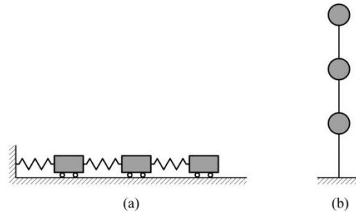
Fig. 5 Equivalent models for calculating storey stiffness; (a) Shear model, (b) Flexural model
