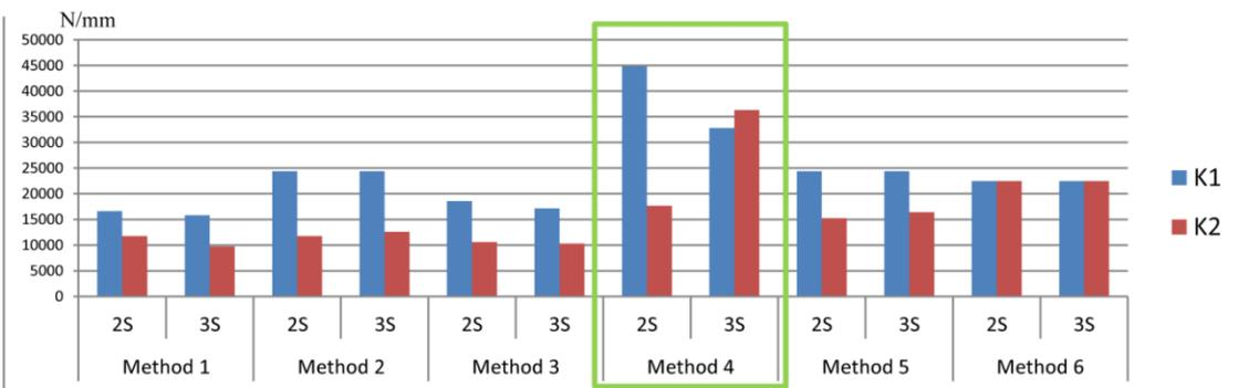
Fig. 13 Comparison between the stiffness of first and second storey in three-storey and two-storey frames with width and Young's modulus of beams equal to columns and rigid supports
