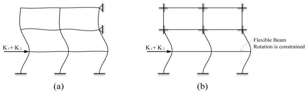
Fig. 18 Finite element model for calculating the storey stiffness; (a) Engineering finite element model, (b) Real finite element model
