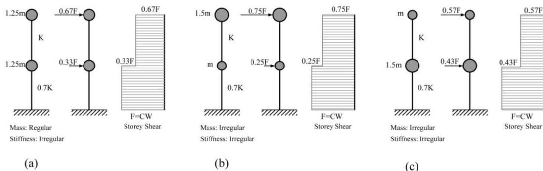
Fig. 6 Effect of mass distribution on intensification of soft storey in buildings with stiffness irregularity; (a) Regular mass distribution, (b) Irregular mass distribution, more mass on top storey, (c) Irregular mass distribution, more mass on bottom storey
