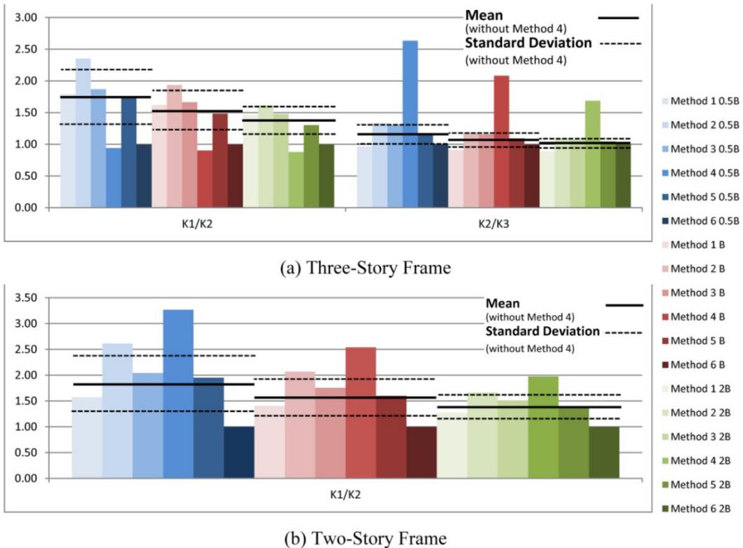
Fig. 15 The storey stiffness to the next storey stiffness for frames with width and Young’s modulus of beams equal to columns and rigid supports; (a) Three-storey frame, (b) Two-storey frame
