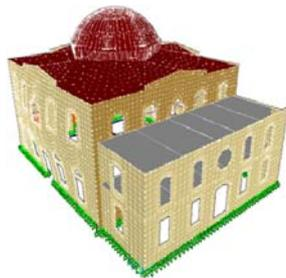
Fig. 11 First mode of the Church in  $X$  direction
