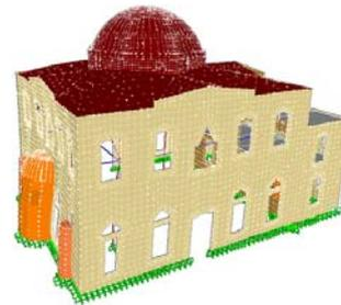
Fig. 12 First mode of the Church in  $Y$  direction
