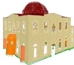
Fig. 14 First mode of the Church in  $Y$  direction considering SSI effects
