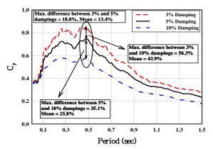
Fig. 7 Sensitivity of constant damage spectrum to damping ratio
