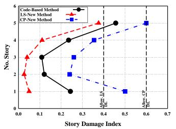
Fig. 13 Comparison between story level damage index of different design methods and performance levels
