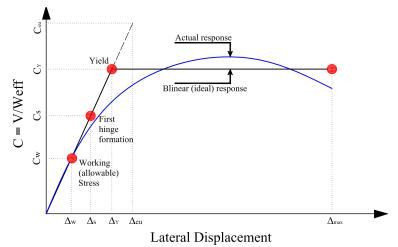
Fig. 3 Schematic relation between elastic and real response of structure
