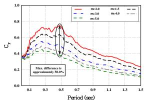
Fig. 6 Sensitivity of constant damage spectrum to ductility
