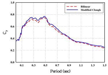
Fig. 8 Sensitivity of the constant damage spectrum to the employed hysteresis model
