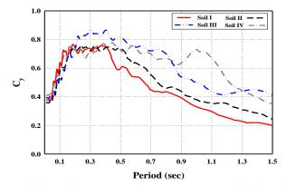
Fig. 9 Sensitivity of the constant damage spectrum to the site soil type
