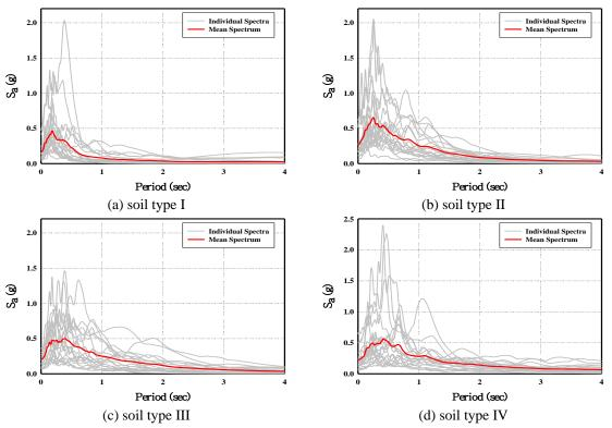
Fig. 4 damped (5%) elastic spectrum of selected ground motion records
