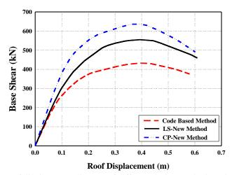
Fig. 12 Base shear- roof displacement diagram of different design methods and performance levels
