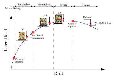
Fig. 1 Shematic relation between building performance and damage states
