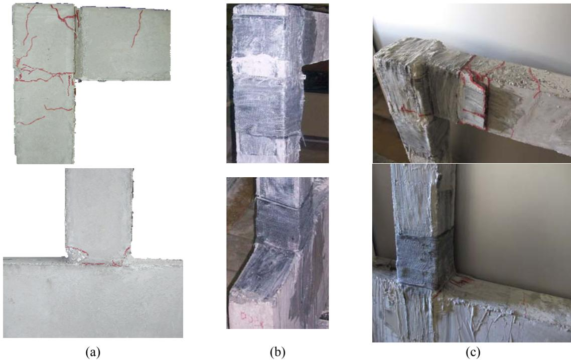
Fig. 7 (a) Joint regions cracking configuration of original specimen F; (b) The applied repair procedure with sheets; (c) Joint regions cracking configuration of repaired specimen RF
