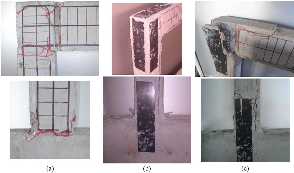
Fig. 6 (a) Joint regions cracking configuration of original specimen B; (b) The applied repair procedure with strips; (c) Joint regions cracking configuration of repaired specimen RB
