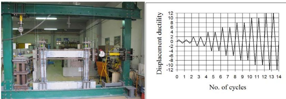
Fig. 2 Test setup of specimen RF and loading program
