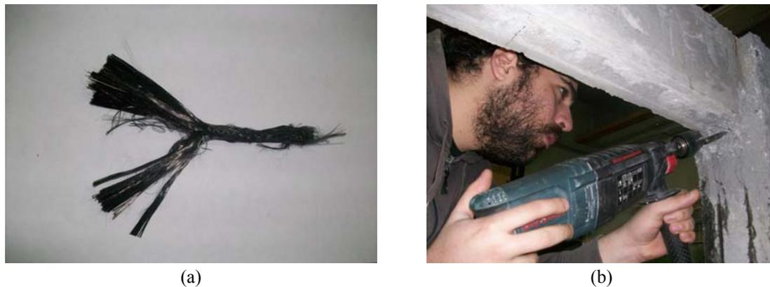
Fig. 5 (a) Construction of CFRP anchors; (b) location of CFRP anchors in Specimen F
