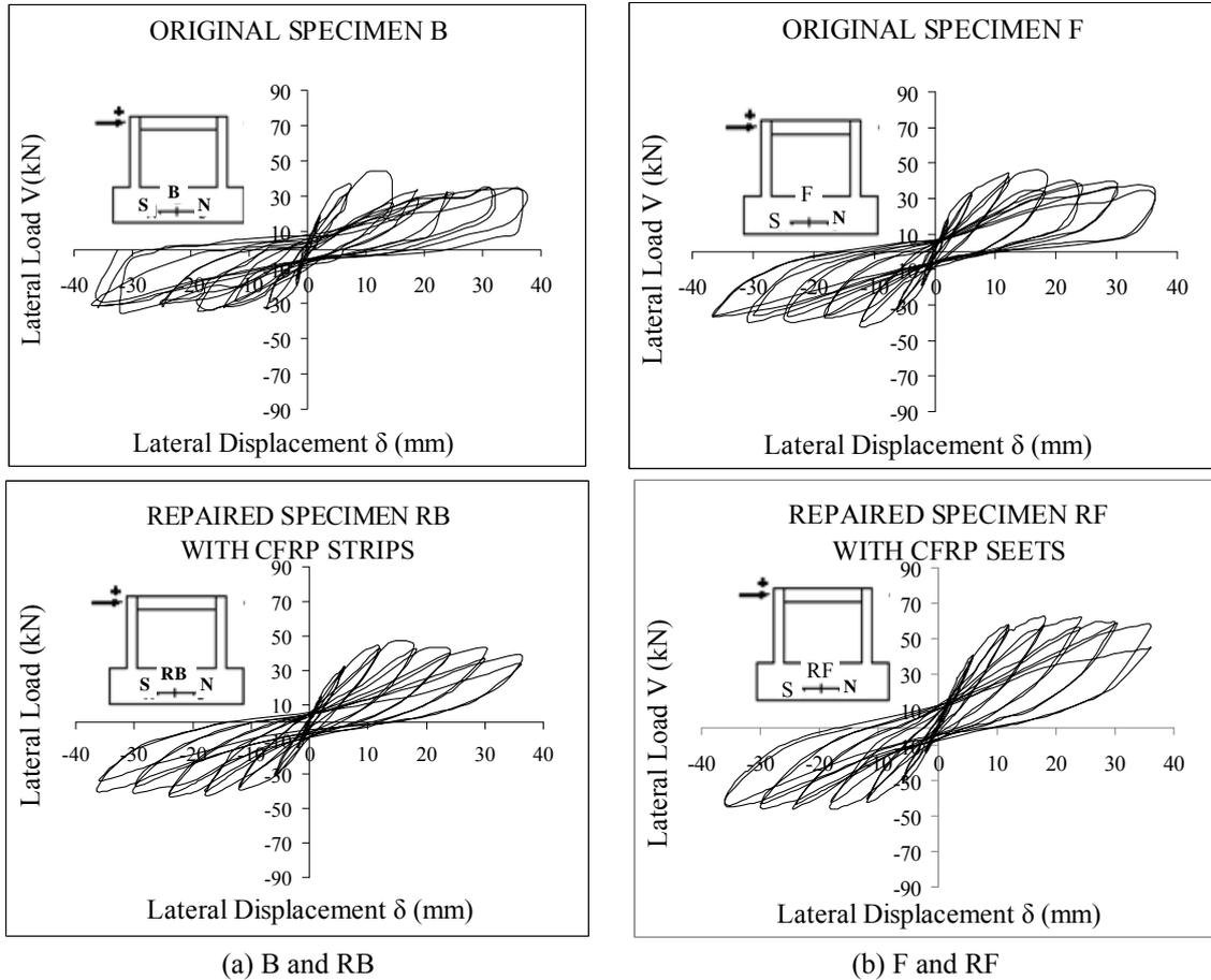
Fig. 8 Load - Displacement hysteresis curves of original and repaired specimens
