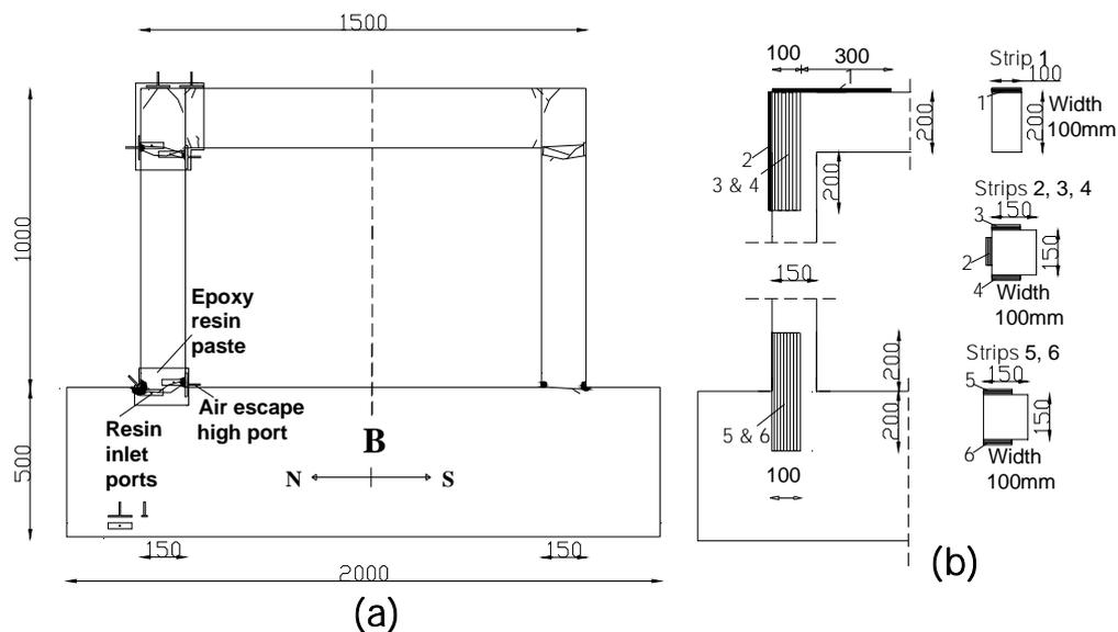
Fig. 3 (a) Application of epoxy injections; (b) arrangement and location of CFRP strips in Specimen B (units in mm)
