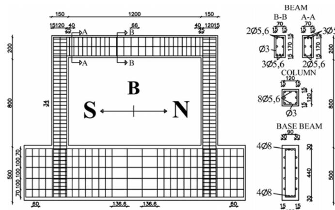
Fig. 1 Reinforcement detailing of the RC frame models (mm)
