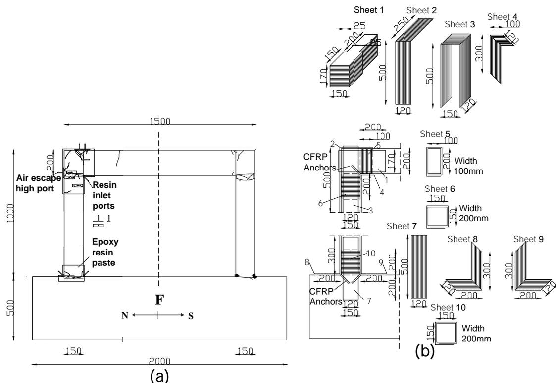
Fig. 4 (a) Application of epoxy injections; (b) arrangement and location of CFRP sheets in Specimen F (units in mm)
