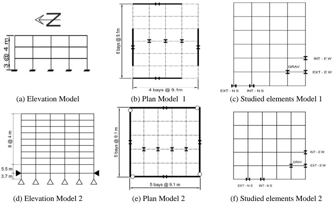
Fig. 1 Elevation, plan and element location for Models 1 and 2
