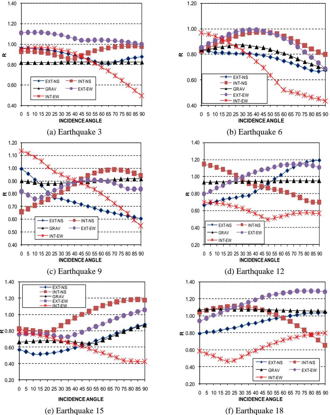
Fig. 3 Ratio (R) of axial load of rotated components to that of principal components, Model 1 and elastic behavior
