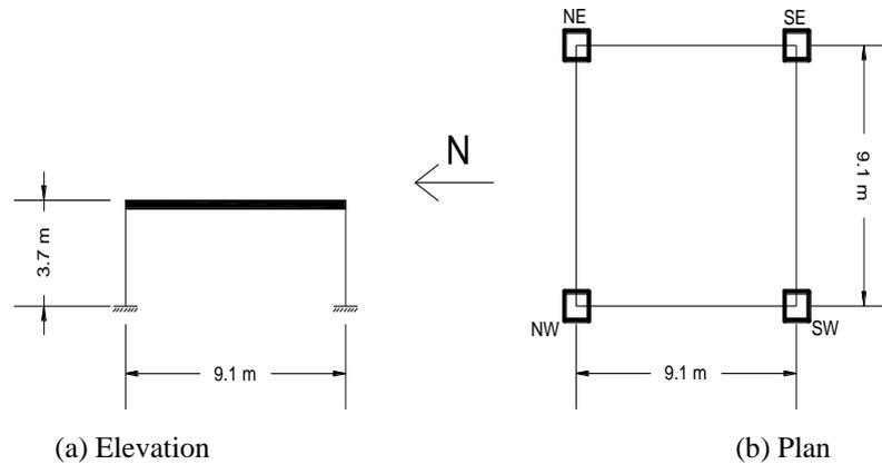
Fig. 2 Elevation and plan of the equivalent SDOF models (Models 1E and 2E)
