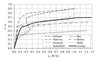
Fig. 8 Curves for relative top displacement (u/H), DCM RC wall
