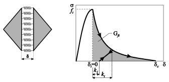
Fig. 4 Strain softening curve defined in terms of displacements
