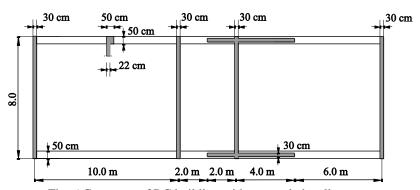
Fig. 6 Geometry of RC building with uncoupled wall system
