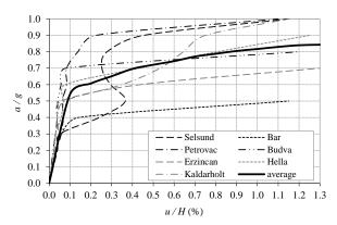
Fig. 9 Curves for relative top displacement (u/H), DCH RC wall
