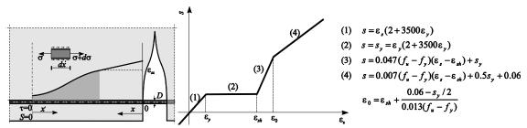
Fig. 5 Discrete crack and steel strain-slip relation under monotonic loading
