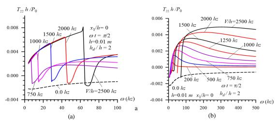
Fig. 7 Frequency response of  $T_{22}h/P_0$  under h = 0.01m,  $h_d/h = 2$ ,  $\omega t = \pi/2$  and  $x_1/h = 0$  for various values of the plate moving velocity V/h in the cases where  $4hz \le \omega \le 100hz$  (a) and  $\omega_{cr} < \omega' \le \omega \le 500hz$  (b)
