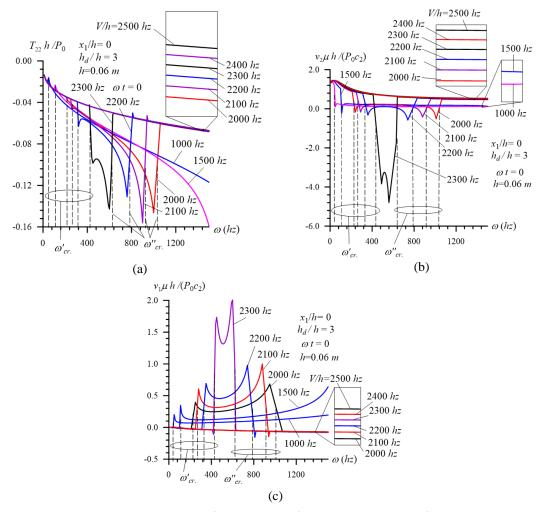
Fig. 15 Frequency response of  $T_{22}h/P_0$  (a),  $v_2\mu h/(P_0c_2)$  (b) and  $v_1\mu h/(P_0c_2)$  (c) and critical frequencies  $\omega'_{cr}$  and  $\omega''_{cr}$  for various values of V/h in the case where h = 0.06m,  $\omega t = 0$ ,  $h_d/h = 2$  and  $x_1/h = 0$  under  $4hz \le \omega \le 1500hz$
