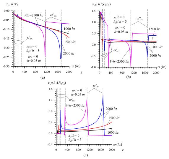
Fig. 14 Frequency response of  $T_{22}h/P_0$  (a),  $v_2\mu h/(P_0c_2)$  (b) and  $v_1\mu h/(P_0c_2)$  (c) and critical frequencies  $\omega'_{cr}$  and  $\omega''_{cr}$  for various values of V/h in the case where h = 0.05m,  $\omega t = 0$ ,  $h_d/h = 2$  and  $x_1/h = 0$  under  $4hz \le \omega \le 2000hz$
