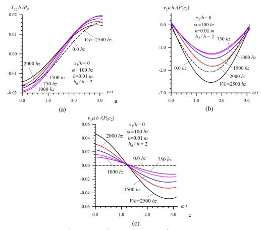
Fig. 10 Dependence of  $T_{22}h/P_0$  (a),  $v_2\mu h/(P_0c_2)$  (b) and  $v_1\mu h/(P_0c_2)$  (c) on the frequency phase  $\omega t$  for various values of the plate moving velocity V/h under  $\omega = 100hz$ , h = 0.01m,  $h_d/h = 2$  and  $x_1/h = 0$
