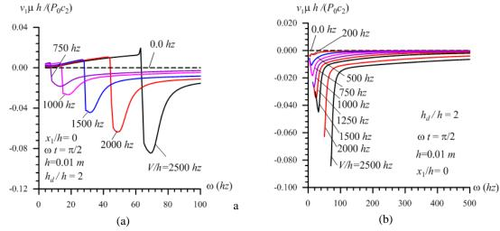
Fig. 4 The influence of the plate moving velocity on the frequency response of the dimensionless velocity  $v_1 \mu h / (P_0 c_2)$  in the cases where  $4h_z \le \omega \le 100 h_z$  (a) and  $\omega_{cr} < \omega' \le \omega \le 500 h_z$  (b)
