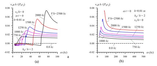
Fig. 9 Frequency response of  $v_1\mu h/(P_0c_2)$  under h = 0.01m,  $h_d/h = 2$ ,  $\omega t = 0$  and  $x_1/h = 0$  for various values of the plate moving velocity V/h in the cases where  $4hz \le \omega \le 100hz$  (a) and  $\omega_{cr} < \omega' \le \omega \le 500hz$  (b)
