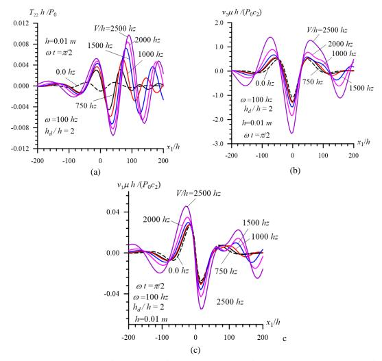
Fig. 17 Distribution of  $T_{22}h/P_0$  (a),  $v_2\mu h/(P_0c_2)$  (b) and  $v_1\mu h/(P_0c_2)$  (c) with respect to  $x_1/h$  for various values of the plate moving velocity V/h in the case where  $\omega t = \pi/2$ ,  $\omega = 100 hz$ , h = 0.01m and  $h_d/h = 2$
