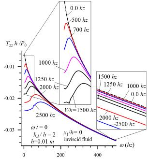
Fig. 5 The influence of the plate moving velocity on the frequency response of the dimensionless stress  $T_{22}h/P_0$  in the case where the fluid is modeled as inviscid
