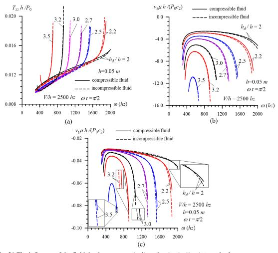
Fig. 21 The influence of the fluid depth parameter  $h_d/h$  under  $2 \le h_d/h \le 3.5$  on the frequency response of  $T_{22}h/P_0$  (a),  $v_2\mu h/(P_0c_2)$  (b) and  $v_1\mu h/(P_0c_2)$  (c), on  $\omega'_{cr}$  and  $\omega''_{cr}$ , and on the effect of the fluid compressibility on this influence in the case where h = 0.05m, V/h = 2500hz,  $\omega t = \pi/2$  and  $x_1/h = 0$
