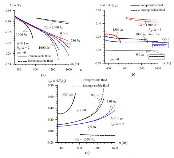
Fig. 20 The influence of the fluid compressibility on the frequency response of  $T_{22}h/P_0$  (a),  $v_2\mu h/(P_0c_2)$  (b) and  $v_1\mu h/(P_0c_2)$  (c) for various values of the plate moving velocity V/h in the case where h = 0.1m,  $h_d/h = 2$ ,  $\omega t = 0$  and  $x_1/h = 0$
