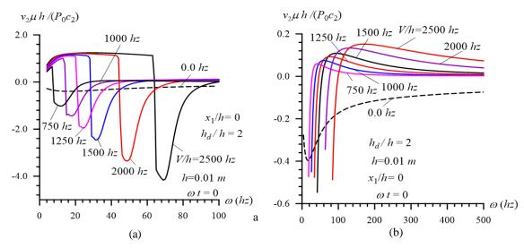
Fig. 8 Frequency response of  $v_2\mu h/(P_0c_2)$  under h = 0.01m,  $h_d/h = 2$ ,  $\omega t = 0$  and  $x_1/h = 0$  for various values of the plate moving velocity V/h in the cases where  $4hz \le \omega \le 100hz$  (a) and  $\omega_{cr} < \omega' \le \omega \le 500hz$  (b)
