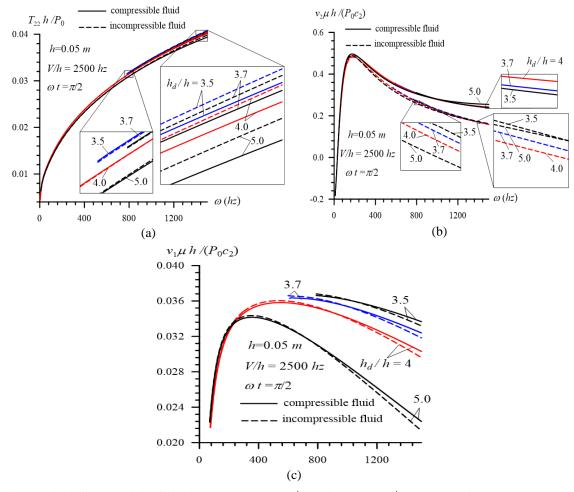
Fig. 22 The influence of the fluid depth parameter  $h_d/h$  under  $3.5 \le h_d/h \le 5$  on the frequency response of  $T_{22}h/P_0$  (a),  $v_2\mu h/(P_0c_2)$  (b) and  $v_1\mu h/(P_0c_2)$  (c), on  $\omega'_{cr}$  and  $\omega''_{cr}$ , and on the effect of the fluid compressibility on this influence in the case where h = 0.05m, V/h = 2500hz,  $\omega t = \pi/2$  and  $x_1/h = 0$
