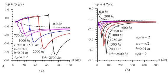
Fig. 3 The influence of the plate moving velocity on the frequency response of the dimensionless velocity  $v_2\mu h/(P_0c_2)$  in the cases where  $4hz \le \omega \le 100hz$  (a) and  $\omega_{cr} < \omega' \le \omega \le 500hz$  (b)
