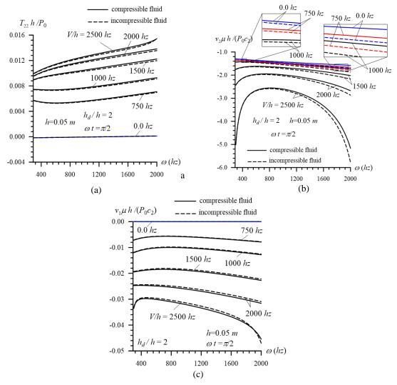
Fig. 19 The influence of the fluid compressibility on the frequency response of  $T_{22}h/P_0$  (a),  $v_2\mu h/(P_0c_2)$ (b) and  $v_1\mu h/(P_0c_2)$  (c) for various values of the plate moving velocity V/h in the case where h = 0.05m,  $h_d/h = 2$ ,  $\omega t = \pi/2$  and  $x_1/h = 0$
