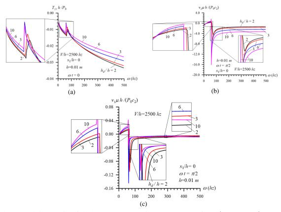
Fig. 12 The influence of the fluid depth  $h_d / h$  on the frequency response of  $T_{22}h/P_0$  (a),  $v_2\mu h/(P_0c_2)$  (b) and  $v_1\mu h/(P_0c_2)$  (c), and on the critical frequency  $\omega_{cr}$  in the case where V/h = 2500hz,  $\omega t = 0$ , h = 0.01m and  $x_1/h = 0$
