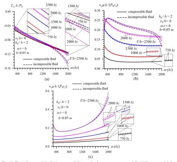
Fig. 18 The influence of the fluid compressibility on the frequency response of  $T_{22}h/P_0$  (a),  $v_2\mu h/(P_0c_2)$ (b) and  $v_1\mu h/(P_0c_2)$  (c) for various values of the plate moving velocity V/h in the case where h = 0.05m,  $h_d/h = 2$ ,  $\omega t = 0$  and  $x_1/h = 0$
