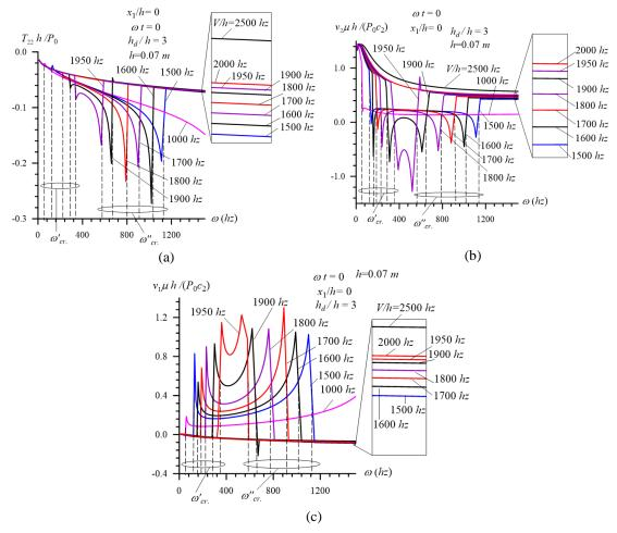
Fig. 16 Frequency response of  $T_{22}h/P_0$  (a),  $v_2\mu h/(P_0c_2)$  (b) and  $v_1\mu h/(P_0c_2)$  (c) and critical frequencies  $\omega'_{cr}$  and  $\omega''_{cr}$  for various values of V/h in the case where h = 0.07m,  $\omega t = 0$ ,  $h_d/h = 2$  and  $x_1/h = 0$  under  $4hz \le \omega \le 1500hz$
