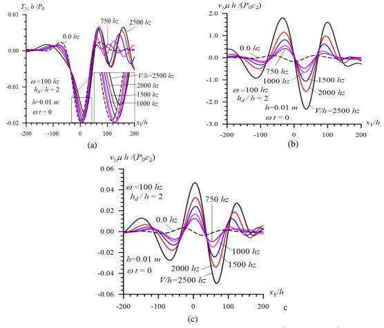
Fig. 6 The influence of the plate moving velocity on the distribution of  $T_{22}h/P_0$  (a),  $v_2\mu h/(P_0c_2)$  (b) and  $v_1\mu h/(P_0c_2)$ ) (c) with respect to  $x_1/h$
