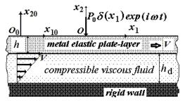
Fig. 1 Sketch of the hydro-elastic system under consideration
