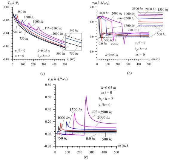
Fig. 13 Frequency response of  $T_{22}h/P_0$  (a),  $v_2\mu h/(P_0c_2)$  (b) and  $v_1\mu h/(P_0c_2)$  (c) and critical frequencies  $\omega_{cr}$  for various values of V/h in the case where h = 0.05m,  $\omega t = 0$ ,  $h_d/h = 2$  and  $x_1/h = 0$
