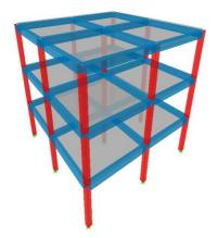
Fig. 4 Mathematical model of frame assuming fixed column bases using ETABS
