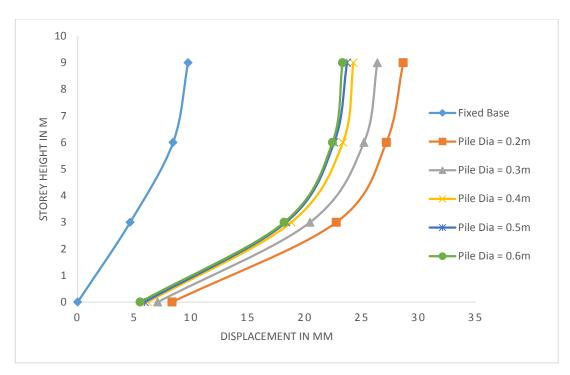
Fig. 6 Effect of pile diameter on displacement
