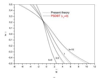
Fig. 2 The variation of the axial displacement  $\overline{u}$  through-the-thickness of a FG beam (L = 2h)
