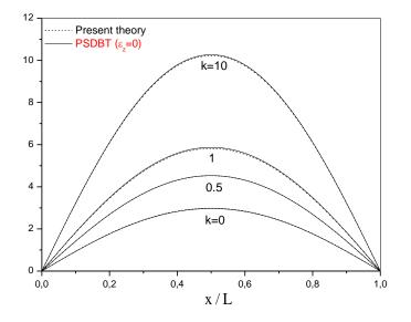
Fig. 5 Variation of the transverse displacement w versus non-dimensional length of a FG beam (L = 5h)
