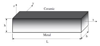
Fig. 1 Geometry and coordinate of a FG beam
