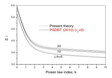
Fig. 6 Variation of the nondimensional fundamental frequency  $\omega$  of FG beam with power law index k and span-to-depth ratio L/h
