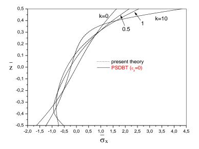
Fig. 3 The variation of the axial stress  $\overline{\sigma}_x$  through-the-thickness of a FG beam (L = 2h)
