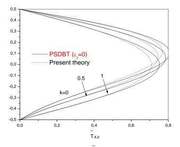
Fig. 4 The variation of the transverse shear stress  $\tau_{xz}$  through-the-thickness of a FG beam (L = 2h)
