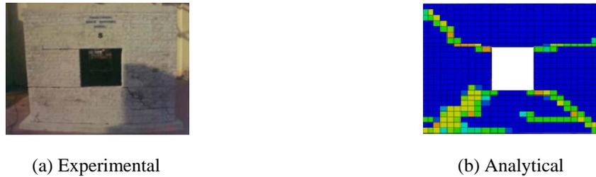
Fig. 16 Comparison of damage on north side wall after fourth shock (Diagonal shear cracks starting from window opening and horizontal cracks at the base of the walls and from the corner of the window opening)
