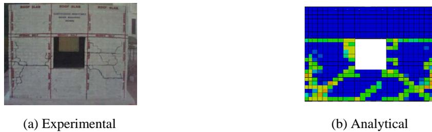
Fig. 19 Comparison of damage on north side wall after seventh shock (Diagonal shear crack were also observed at the corners of the walls)
