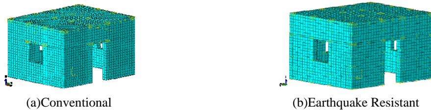
Fig. 4 Meshed finite element of brick masonry building
