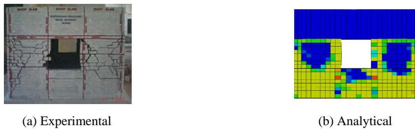
Fig. 20 Comparison of damage on north side wall after eight shock (Several diagonal shear cracks were also observed at north shear wall)
