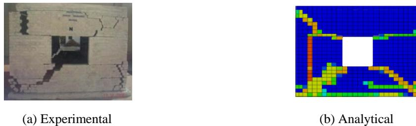
Fig. 17 Comparison of damage on north side wall after fifth shock (Wide and diagonal shear crack originating from window openings and spreading to the corner)
