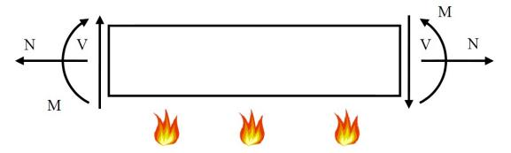
Fig. 1 Mechanical loading and fire acting on reinforced concrete element
