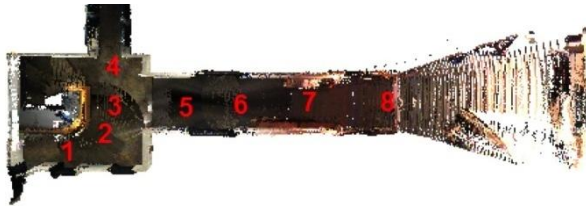
Figure 19. Eight scans aligned to form a complete map of a building hallway with approximately five million points.
