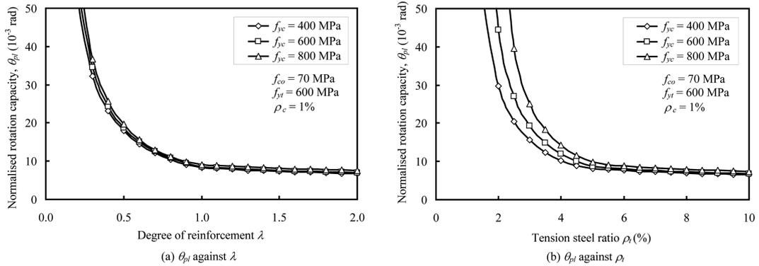
Fig. 5 Effects of compression steel yield strength on deformability
