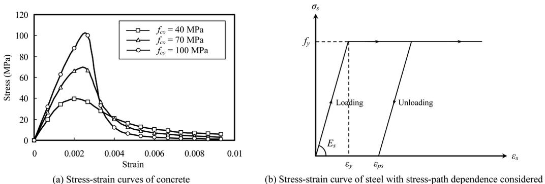
Fig. 1 Stress-strain curves of concrete and steel reinforcement
