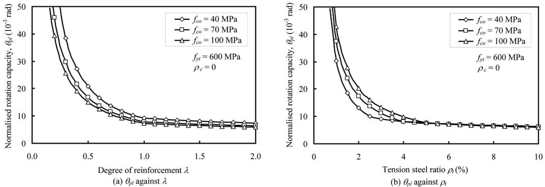
Fig. 3 Variation of deformability with degree of reinforcement and tension steel ratio
