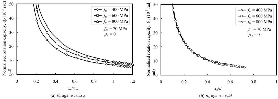
Fig. 7 Variation of  $\theta_{pl}$  of deformability with neutral axis depth at different steel yield strength
