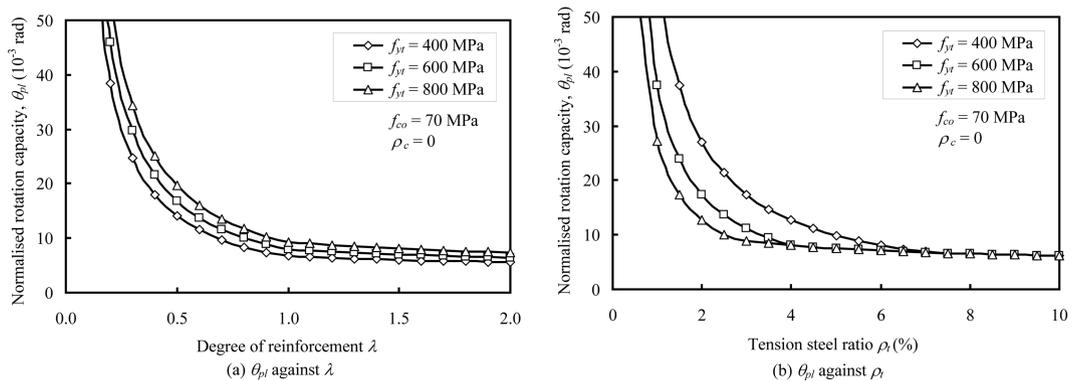
Fig. 4 Effects of tension steel yield strength on deformability
