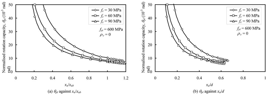
Fig. 6 Variation of deformability with neutral axis depth at different concrete strength
