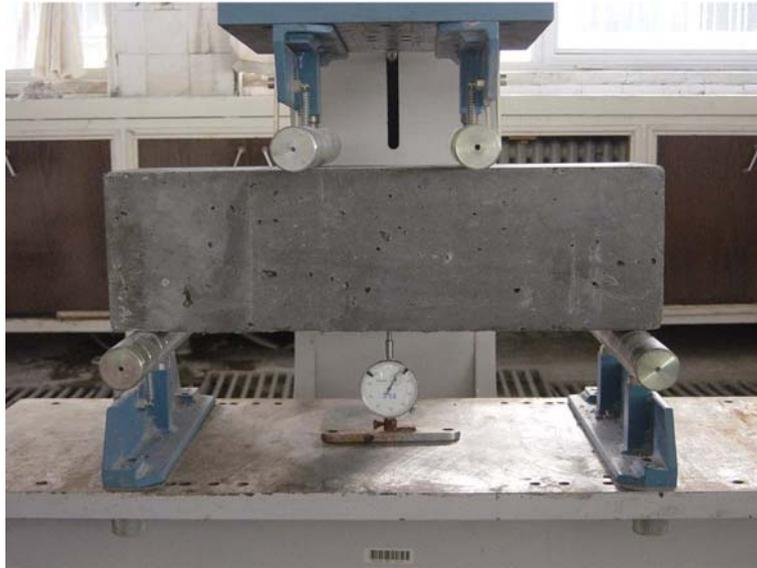
Fig. 2 Testing a concrete prism in flexure
