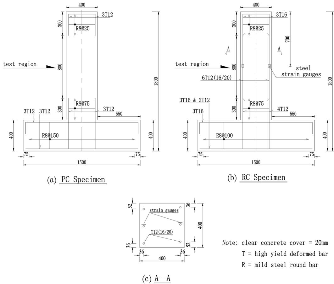
Fig. 2 Details of steel reinforcement
