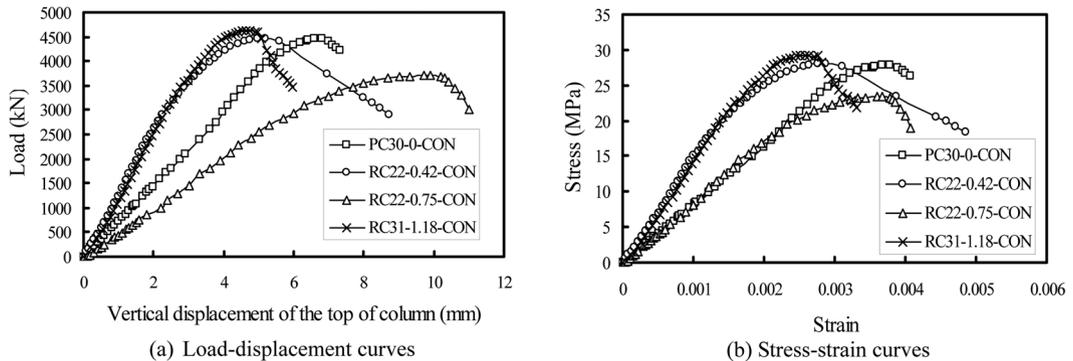
Fig. 7 Load-displacement and stress-strain curves of concrete of concentrically loaded specimens
