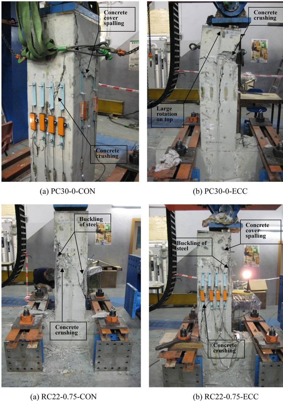
Fig. 6 Some observed behaviour of test specimens after test
