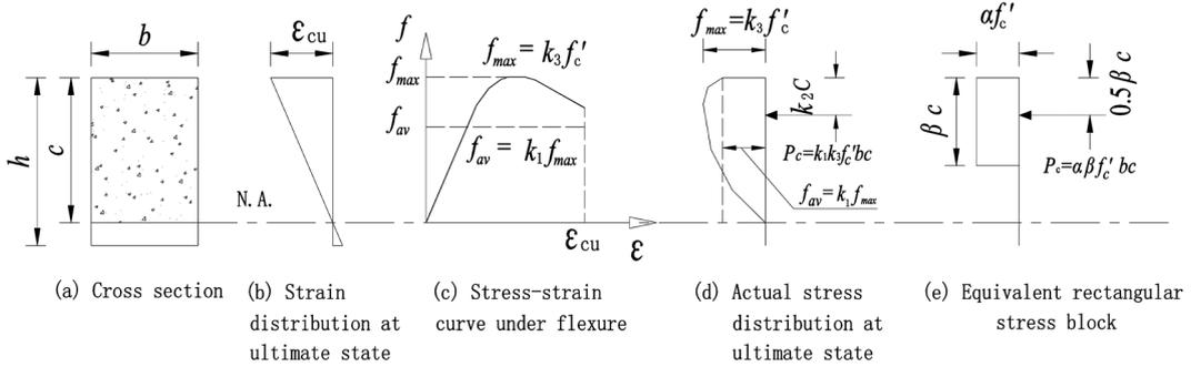
Fig. 1 Concrete stress block parameters
