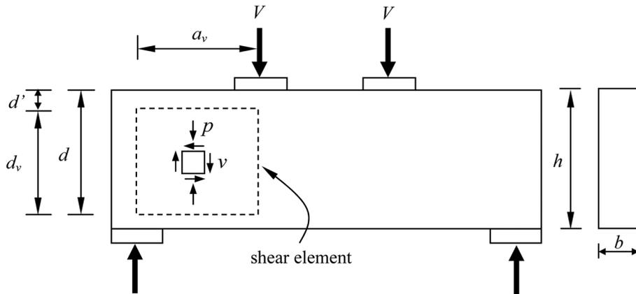
Fig. 4 Concrete stresses within shear span of a deep beam
