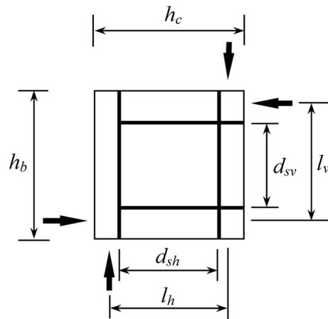
Fig. 6 Dimensions of a beam-column joint
