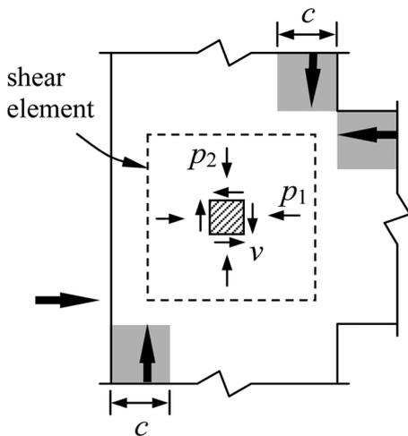
Fig. 5 Stresses in an exterior beam-column joint
