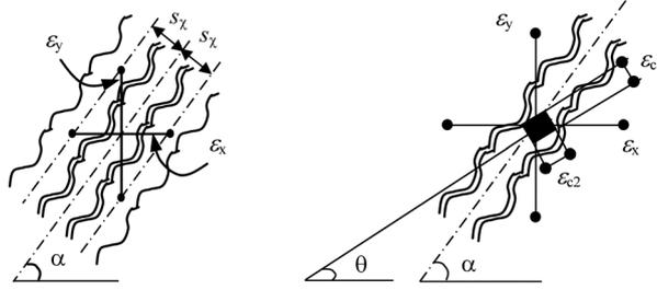
Fig. 3 Strain state of concrete strut
