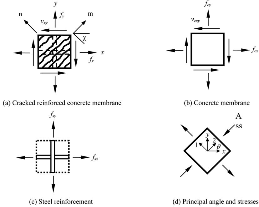
Fig. 1 Stresses of cracked reinforced concrete membrane elements subjected to shear
