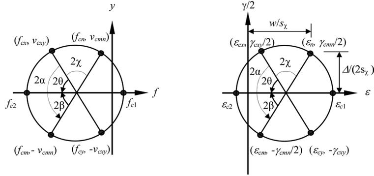
Fig. 2 Mohr circles of average stress and average strain for cracked concrete
