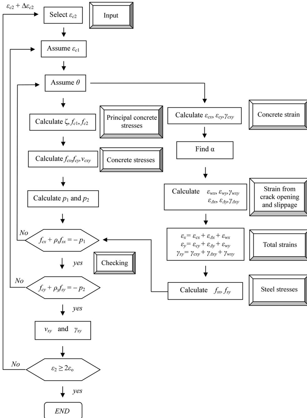
Fig. 7 Flow chart of solution procedure for determining shear stress-strain relationship of beam-column joints by MRA-STM
