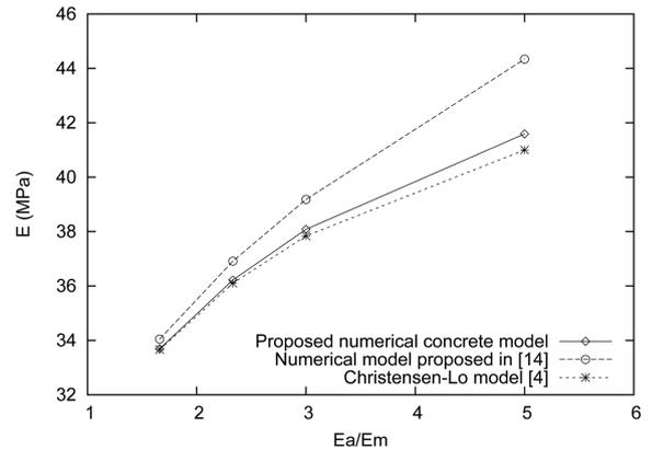
Fig. 4 Two-phase concrete composite: comparison with previous analytical and numerical results
