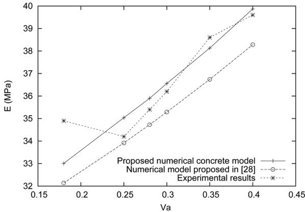
Fig. 3 Two-phase concrete composite: comparison with previous analytical and experimental results
