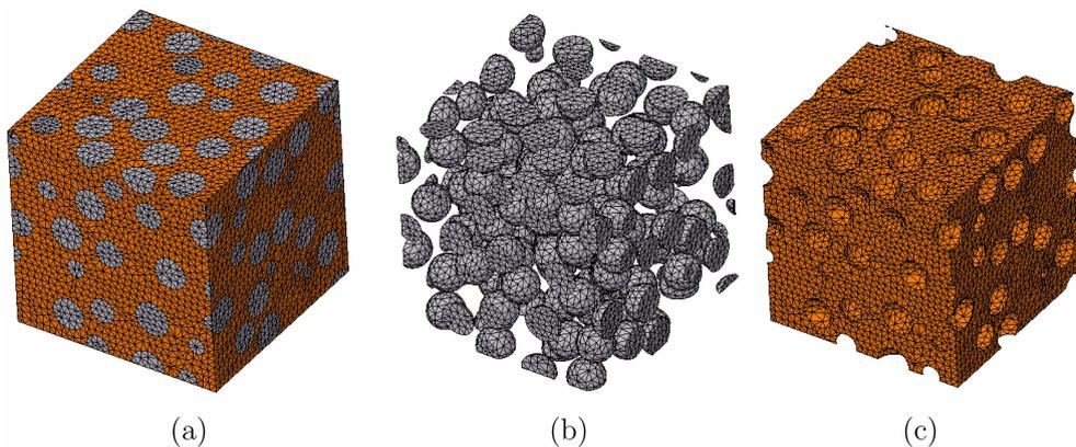
Fig. 2 Finite element models generated for 30% volume fraction of spherical aggregates,  $L = 12$  mm,  $D = 2$  mm,  $s_1 = 0.05r$ ,  $s_2 = 0.05r$ : (a) Complete meshed RVE, (b) Meshed aggregates, (c) Meshed matrix
