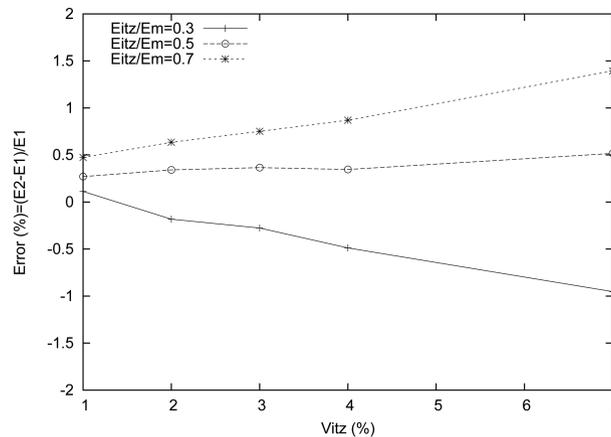
Fig. 8 Evolution of the error between  $E_1$  (numerical model with material discontinuity) and  $E_2$  (second approach of the numerical model). ( $E_a/E_m$ ) = 1.56
