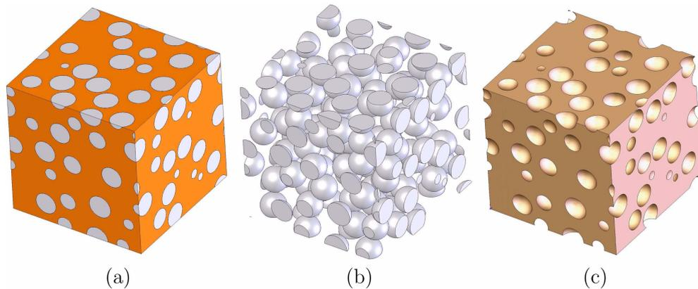
Fig. 1 Unit cell model generated (RVE) for 30% volume fraction of spherical aggregates,  $L = 12$  mm,  $D = 2$  mm,  $s_1 = 0.05r$ ,  $s_2 = 0.05r$ : (a) Complete unit cell, (b) Aggregates, (c) Matrix
