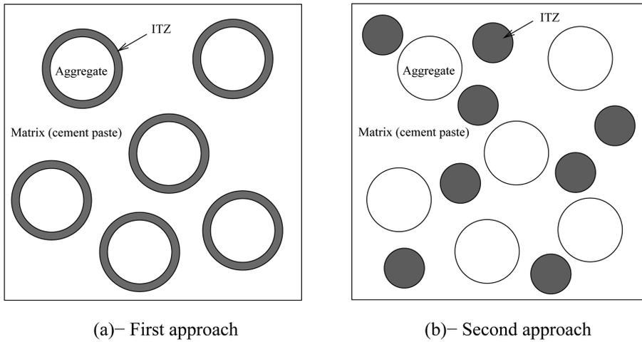
Fig. 5 Numerical concrete composites model with ITZ (conceptual illustrations of 3D models)
