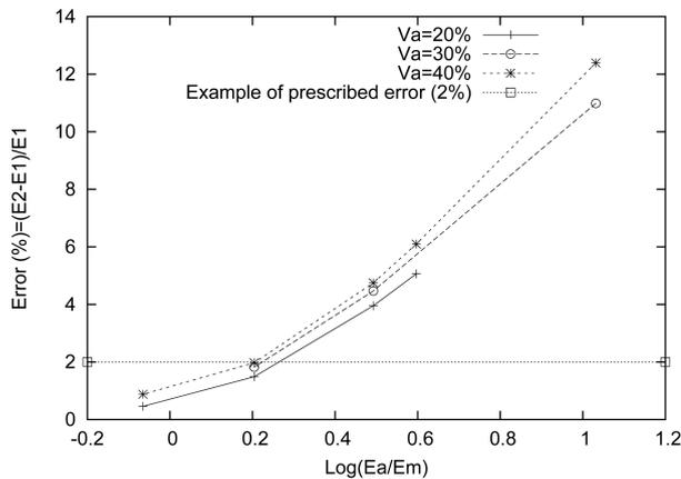
Fig. 7 Evolution of the error between  $E_1$  (analytical model) and  $E_2$  (second approach of the numerical model).  $E_{itz} = 0.5 E_m$
