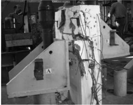
Fig. 6 Failure pattern of EB-1 at ultimate load
