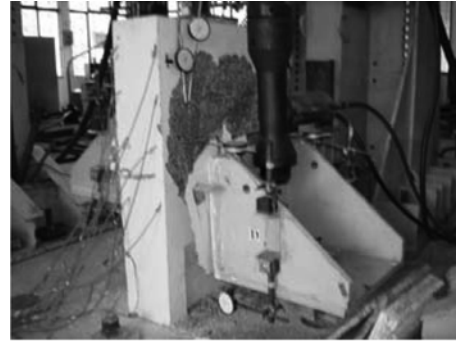
Fig. 7 Failure pattern of EB-4 at ultimate load
