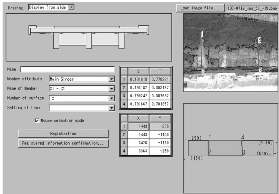
Fig. 3 Sample screen for combining the image with the model
