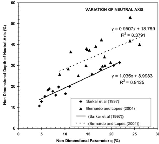
Fig. 3 Variation of neutral axis with geometrical and strength properties of beams
