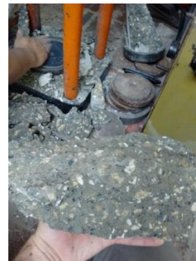
Fig. 5 E-plastic waste concrete cylinder piece after compression test
