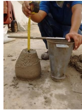
Fig. 4 Slump test of e-plastic waste concrete
