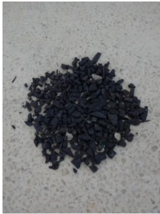
Fig. 2 E-plastic waste aggregate used in this study
