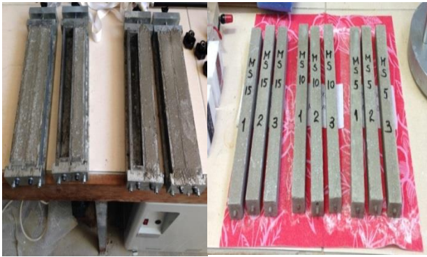
Fig. 2 Mortar bars measuring 25×25×285 mm
