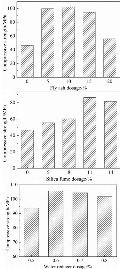
Fig. 5 Influence of fly ash, silica fume and water reducer on compressive strength of hybrid fiber reinforced mortars
