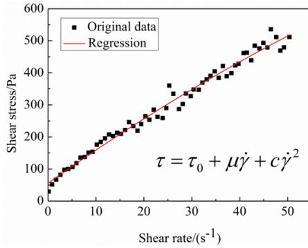
Fig. 4 A typical regression flow curve
