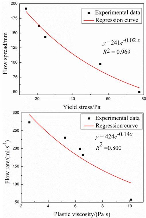
Fig. 9 Correlations between rheological properties and flowability of mortars with various dosage of fly ash
