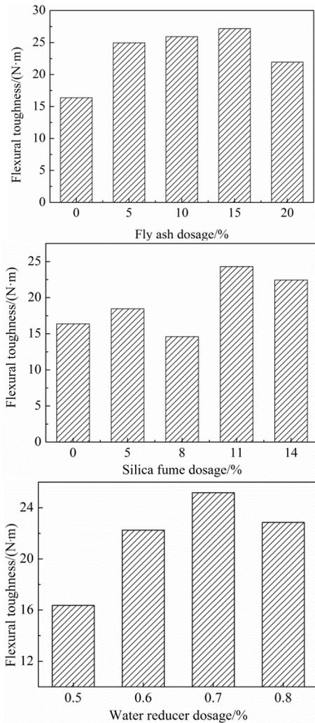
Fig. 8 Influence of fly ash, silica fume and water reducer on flexural toughness of hybrid fiber reinforced mortars
