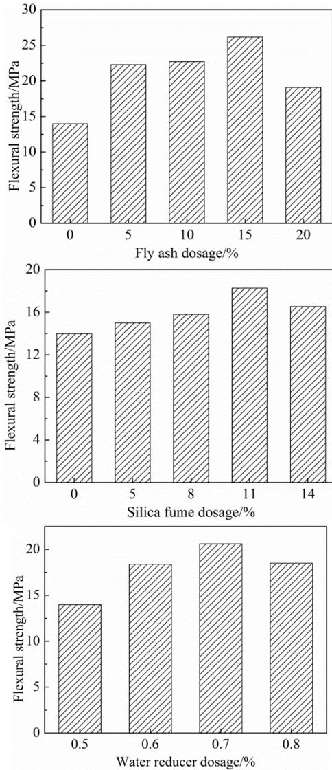
Fig. 6 Influence of fly ash, silica fume and water reducer on flexural strength of hybrid fiber reinforced mortars
