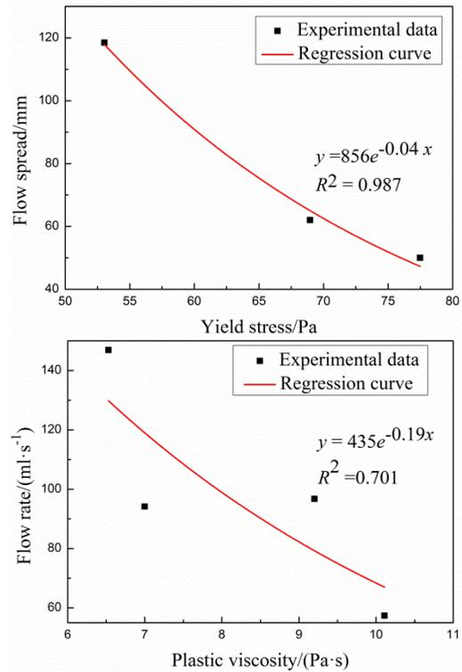
Fig. 10 Correlations between rheological properties and flowability of mortars with various dosage of water reducer. Note: The singular point yield stress=78.0 Pa is given up
