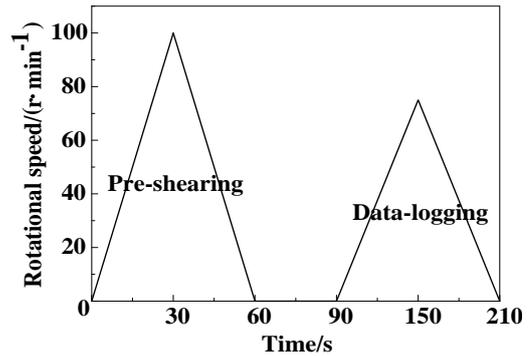
Fig. 2 Procedure of rheological testing
