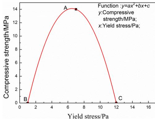
Fig. 12 Typical curve of the mathematical model between rheological and mechanical properties
