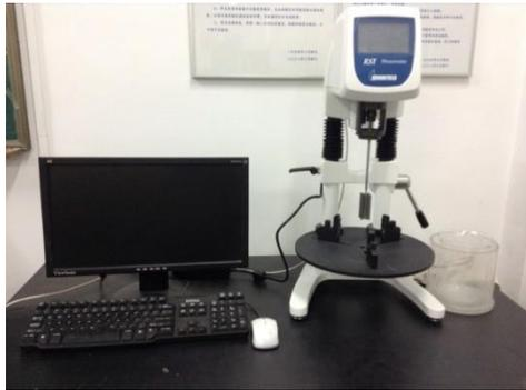
Fig. 1 Equipment for rheological measurement
