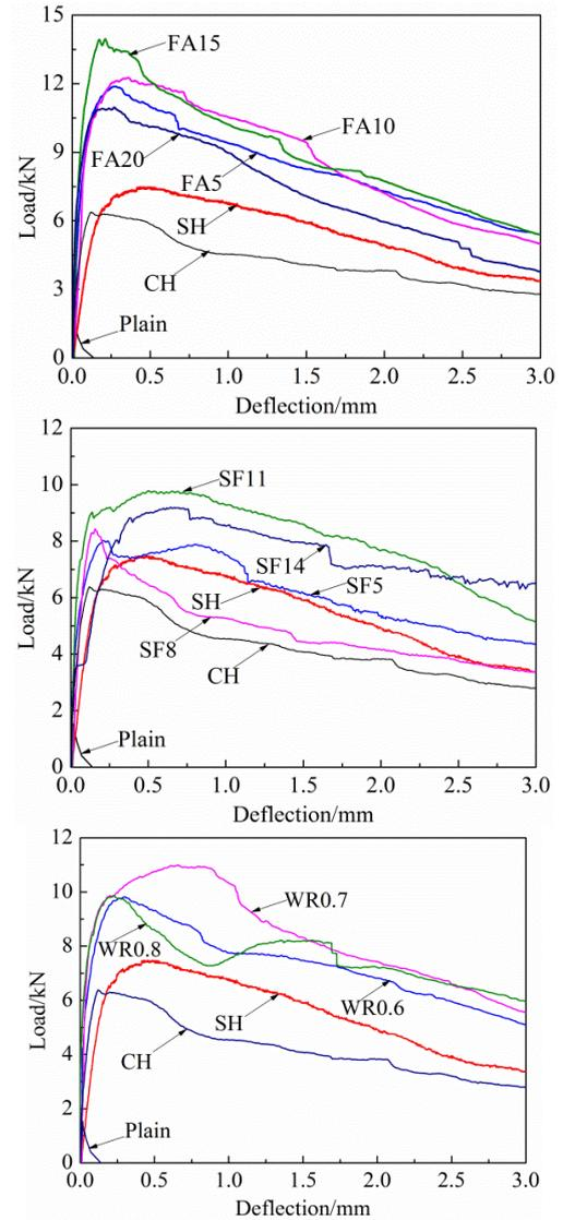
Fig. 7 Load-deflection curves of composites with various dosage of fly ash (FA), silica fume (SF) and water reducer (WR)
