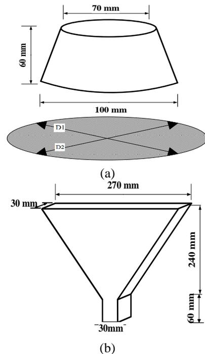
Fig. 3 Schematic graph of (a) slump cone and (b) V funnel (Okamura and Ouchi 2003)
