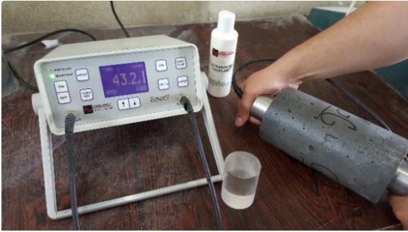
Fig. 4 Ultrasonic pulse velocity testing device and location of transducer placement on RPC specimen
