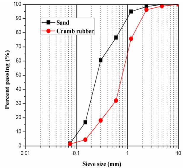
Fig. 1 Gradation of sand and crumb rubber
