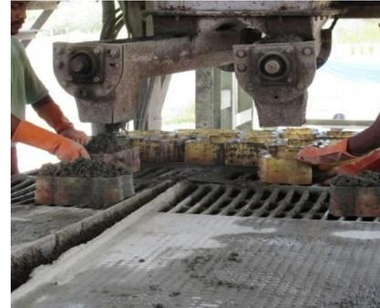
(b) Placing of concrete in PCPB mould
