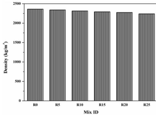
Fig. 3 Density of wet cast PCPB for different crumb rubber content
