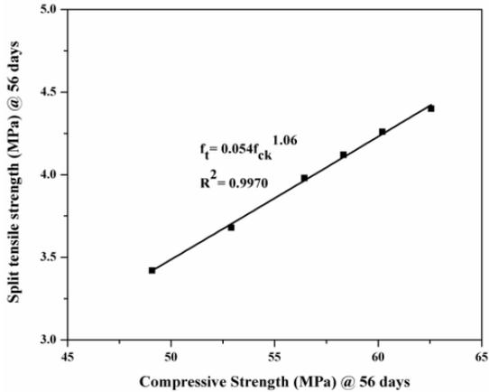
Fig. 11 The Relationship between compressive strength with split tensile strength for wet cast PCPB containing crumb rubber at 56 days
