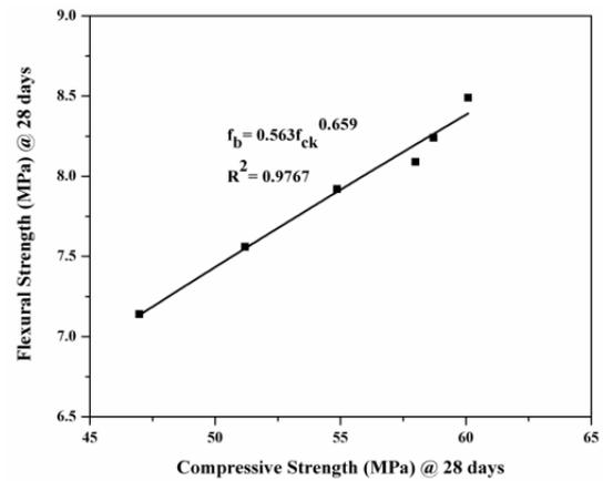
Fig. 10 The Relationship between compressive strength with flexural strength for wet cast PCPB containing crumb rubber at 28 days
