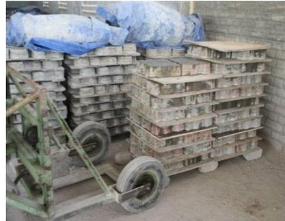
(c) Specimens are arranged for curing
