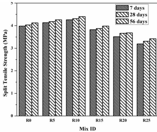
Fig. 5 Split tensile strength of wet cast PCPB for different crumb rubber content
