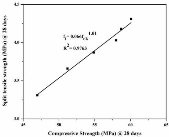
Fig. 9 Relationship between compressive strength with split tensile strength for wet cast PCPB containing crumb rubber at 28 days
