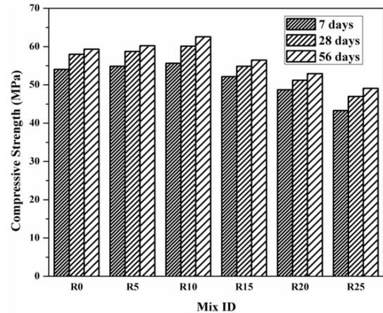
Fig. 4 Compressive strength of wet cast PCPB for different crumb rubber content
