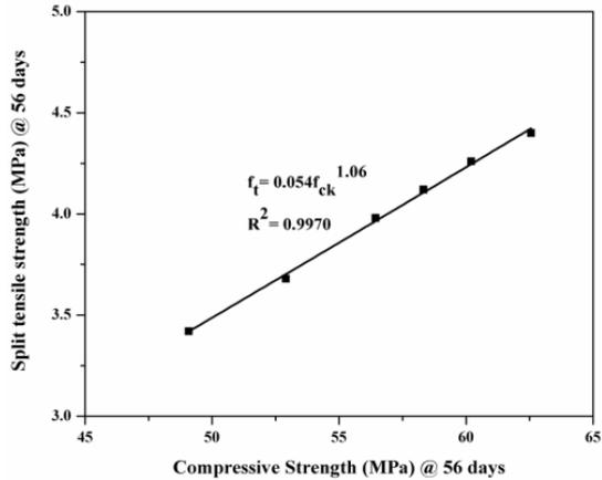
Fig. 11 The Relationship between compressive strength with split tensile strength for wet cast PCPB containing crumb rubber at 56 days
