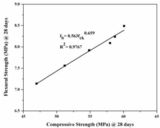
Fig. 10 The Relationship between compressive strength with flexural strength for wet cast PCPB containing crumb rubber at 28 days
