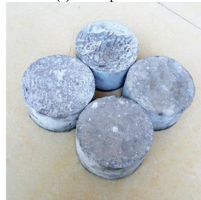
(b) Cylindrical specimens before polish
