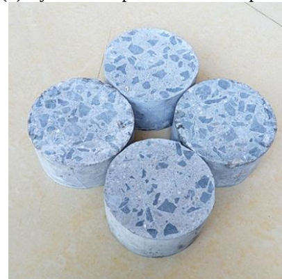
(c) Cylindrical specimens after polish
