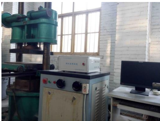
(a) Hydraulically driven test system
