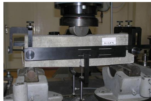
Fig. 5 Displacement controlled flexural 3-point bending test set-up ( V=1.5\% )
